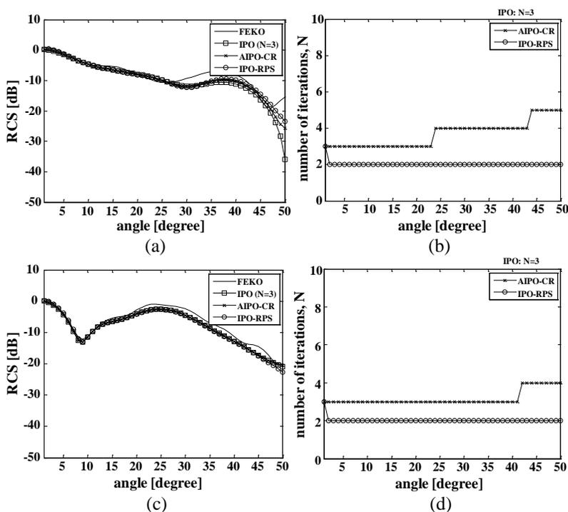
**Figure 3.** Results for the short cylindrical cavity. (a) Monostatic RCS patterns ( $\hat{\phi}$  polarization). (b)  $N(m)$  ( $\hat{\phi}$  polarization). (c) Monostatic RCS patterns ( $\hat{\theta}$  polarization). (d)  $N(m)$  ( $\hat{\theta}$  polarization).
