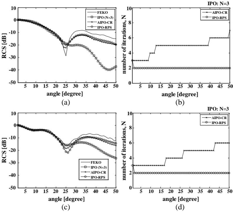
**Figure 4.** Results for the long cylindrical cavity. (a) Monostatic RCS patterns ( $\hat{\phi}$  polarization). (b)  $N(m)$  ( $\hat{\phi}$  polarization). (c) Monostatic RCS patterns ( $\hat{\theta}$  polarization). (d)  $N(m)$  ( $\hat{\theta}$  polarization).
