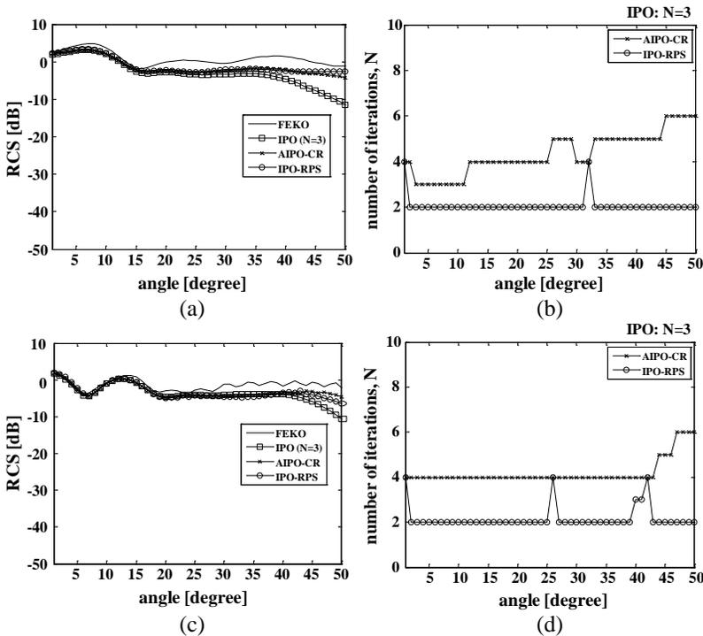
**Figure 6.** Results for the long rectangular cavity. (a) Monostatic RCS patterns ( $\hat{\phi}$  polarization). (b)  $N(m)$  ( $\hat{\phi}$  polarization). (c) Monostatic RCS patterns ( $\hat{\theta}$  polarization). (d)  $N(m)$  ( $\hat{\theta}$  polarization).
