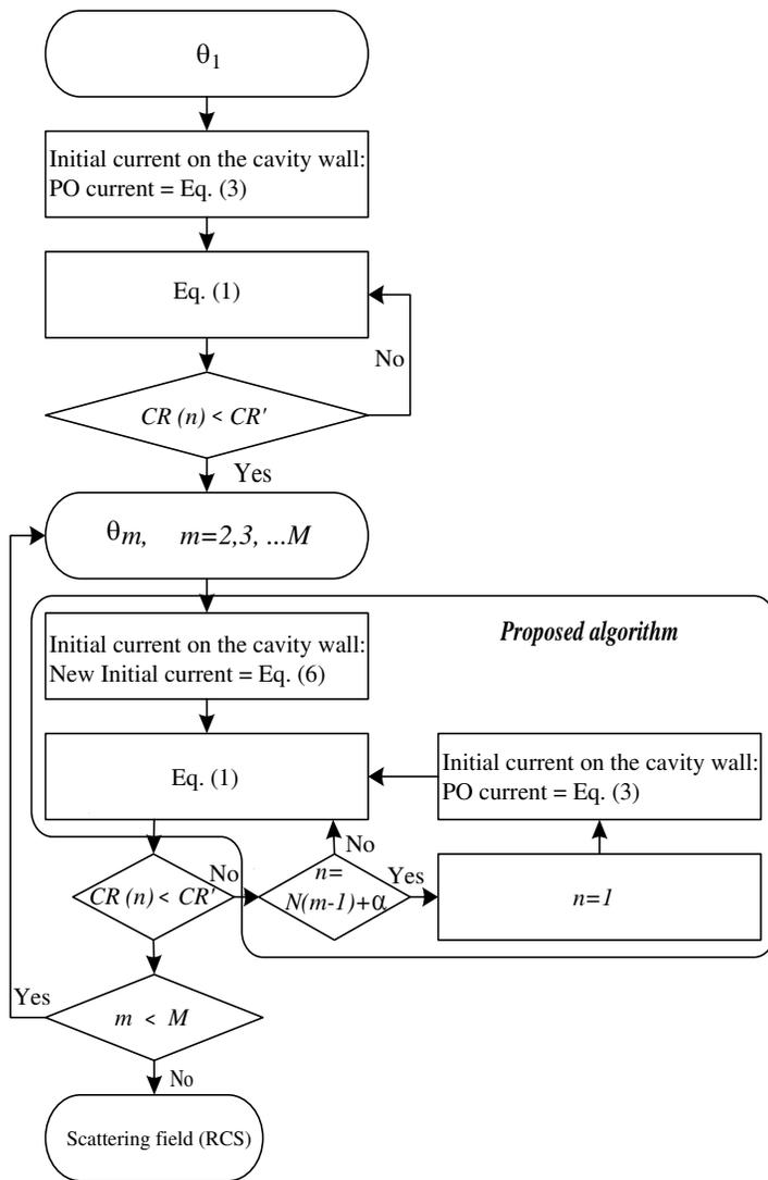
**Figure 1.** Flow chart of the IPO-RPS method.  $CR'$  and  $\alpha$  are predetermined threshold values.
