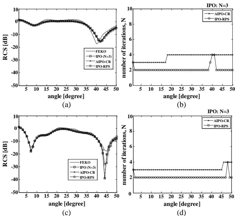
**Figure 5.** Results for the short rectangular cavity. (a) Monostatic RCS patterns ( $\hat{\phi}$  polarization). (b)  $N(m)$  ( $\hat{\phi}$  polarization). (c) Monostatic RCS patterns ( $\hat{\theta}$  polarization). (d)  $N(m)$  ( $\hat{\theta}$  polarization).
