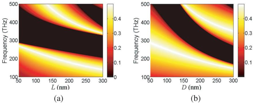
**Figure 5.** Dispersion for the SPPs propagating in slit arrays in  $MDM$  structure. (a) The  $k^{Bloch}L/\pi$  versus frequency and  $L$  with  $D = 200$  nm. (b) The  $k^{Bloch}L/\pi$  versus frequency and  $D$  with  $L = 180$  nm. The black region indicates the photonic stopband. The other structure geometric parameters are  $w_1 = 60$  nm,  $w_2 = 60$  nm, and  $n_B = 1$ .
