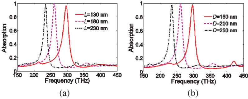
**Figure 6.** Dependence of the absorption spectra on (a)  $L$  when  $D = 200$  nm and (b)  $D$  when  $L = 180$  nm, respectively. The other structure geometric parameters are  $L_m = 14$  nm,  $w_1 = 60$  nm,  $w_2 = 60$  nm,  $N = 3$ ,  $n_A = 1$ , and  $n_B = 1$ .
