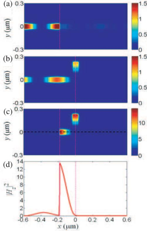
**Figure 4.** Field distributions of  $|H_z|^2$  for the MDM structure at 261.4 THz with (a) single TML and (b) single slit in the MDM core. (c) The  $|H_z|^2$  for the MDM structure at 261.4 THz when the TML and the slit are both inserted in the MDM core. The black dashed line illustrates  $y = 0$   $\mu\text{m}$ . (d) The  $|H_z|^2$  along the  $y = 0$   $\mu\text{m}$ . Here, the left and right perpendicular pink dotted lines represent position of TML interface and slit center, respectively.
