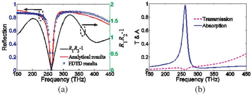
**Figure 3.** (a) Reflection spectrum of the plasmonic absorber and profile of the  $R_1R_2 - 1$ . The red solid line and blue circles represent the reflection obtained by the Eq. (6) and FDTD method, respectively. (b) Transmission and absorption spectra of the plasmonic absorber. The structure geometric parameters are:  $L_m = 14 \text{ nm}$ ,  $L = 180 \text{ nm}$ ,  $D = 200 \text{ nm}$ ,  $w_1 = 60 \text{ nm}$ ,  $w_2 = 60 \text{ nm}$ ,  $N = 1$ ,  $n_A = 1$ , and  $n_B = 1$ .
