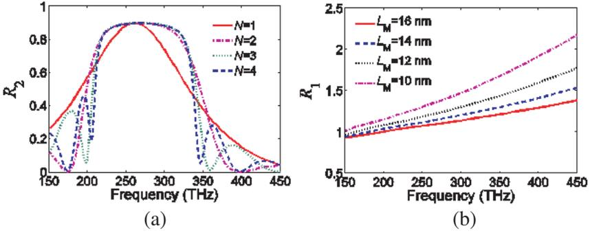
**Figure 2.** (a)  $R_2$  versus frequency with different slit cell  $N$ . (b) Variation of  $R_1$  to frequency and  $L_M$ . The other structure geometric parameters are:  $L = 180$  nm,  $D = 200$  nm,  $w_1 = 60$  nm,  $w_2 = 60$  nm,  $n_A = 1$ , and  $n_B = 1$ .
