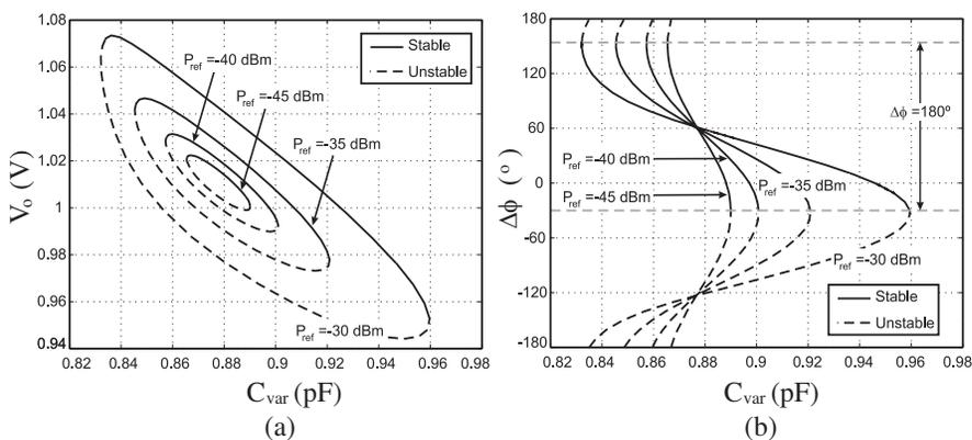
**Figure 3.** Synchronized solutions for different values of  $P_{ref}$ . (a) Amplitude of the autonomous signal. (b) Phase shift evaluated at the fundamental harmonic component of the autonomous signal. Continuous line: Stable solutions. Dashed line: Unstable solutions.
