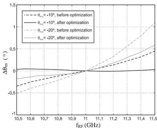
**Figure 13.** Frequency variation of  $\theta_m$  with respect to its value at the center frequency band  $\theta_{m,c}$ . Two cases are considered:  $\theta_{m,c} = -10^\circ$  and  $\theta_{m,c} = -20^\circ$ .
