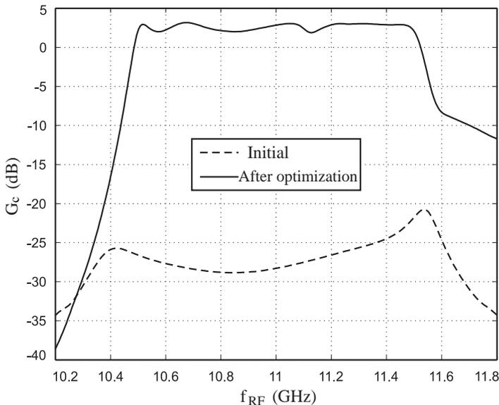
**Figure 2.** Conversion gain of the IL3HSOM. Dashed line: Initial conversion gain, with  $V_o = 1.1$  V and  $V_o^3 = 25$  mV. Continuous line: Conversion gain after setting the operation regime close to three Hopf bifurcation points.
