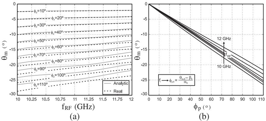
**Figure 8.** (a) Dependence of  $\theta_m$  with the frequency of the input RF signal. Continuous line: Real variation, calculated through electromagnetic simulations. Dashed line: Theoretical variation due to the array factor, given by (3). (b) Variation of  $\theta_m$  versus  $\phi_p$ , evaluated for several frequency points  $f_i$ .
