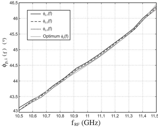
**Figure 11.** Frequency response of the progressive phase shift  $\phi_{p,i}(f)$ , reached between the IF signals of each pair of circuits, after the optimization process.
