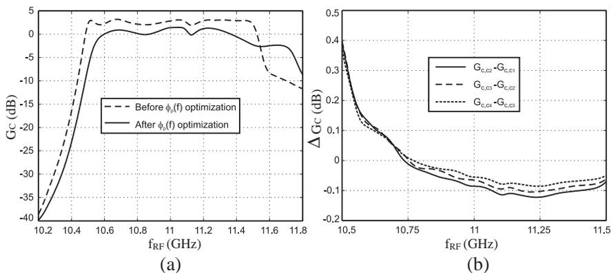
**Figure 12.** Conversion gain after  $\phi_p(f)$  optimization. (a) Frequency response of the conversion gain. (b) Difference between the conversion gain of each pair of adjacent circuits, evaluated at  $f_{RF} = 11$  GHz.
