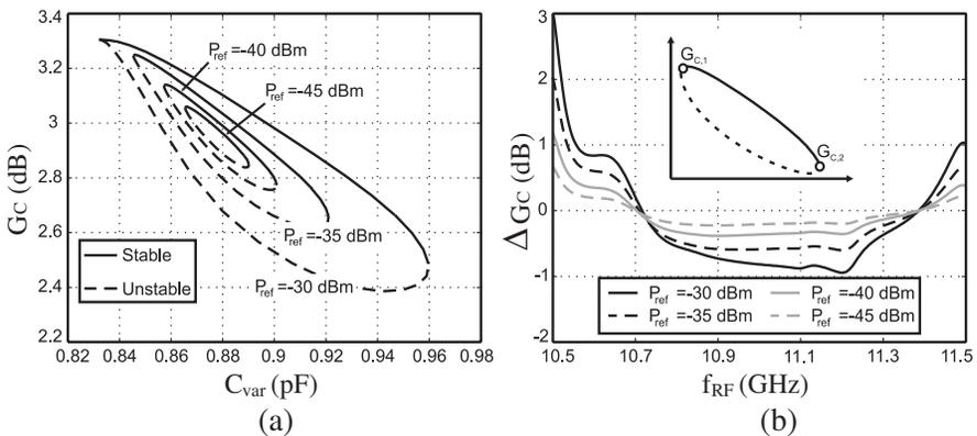
**Figure 5.** (a) Conversion gain, evaluated at  $f_{\text{RF}} = 11$  GHz, along the synchronization loci. Stable solutions are represented with continuous line. (b) Difference between the conversion gain evaluated at the limits of the locking range  $\Delta G_c = G_{c,2} - G_{c,1}$ .
