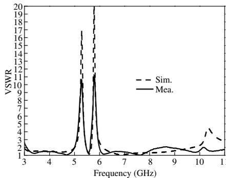
**Figure 4.** Simulated and measured VSWR versus frequency.
