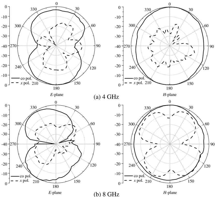
**Figure 8.** Measured radiation patterns at different frequencies.
