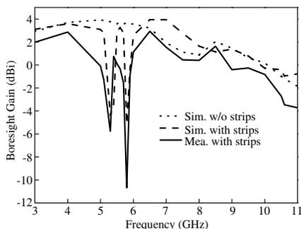
**Figure 9.** Measured realized antenna gain versus frequency.
