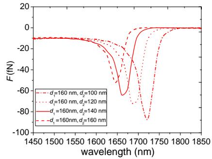
**Figure 8.**  $\vec{F}$  acting on the nanoparticles ( $R_p = 80$  nm and  $\varepsilon_p = 2.25$ ), 180 nm above the MDM fishnet metamaterials at different value of  $d_1, d_2$  as shown in the inset.
