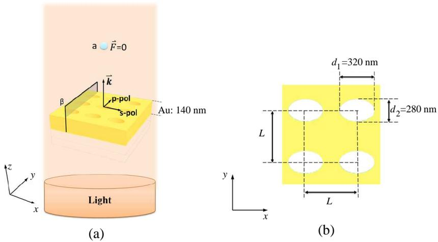
**Figure 5.** (a) schematic of ENA embedded through a single Au layer. The lattice constant is  $L = 680$  nm and hole diameters are  $d_1 = 320$  nm and  $d_2 = 280$  nm. (b) Illustration of the square lattice of ENA.
