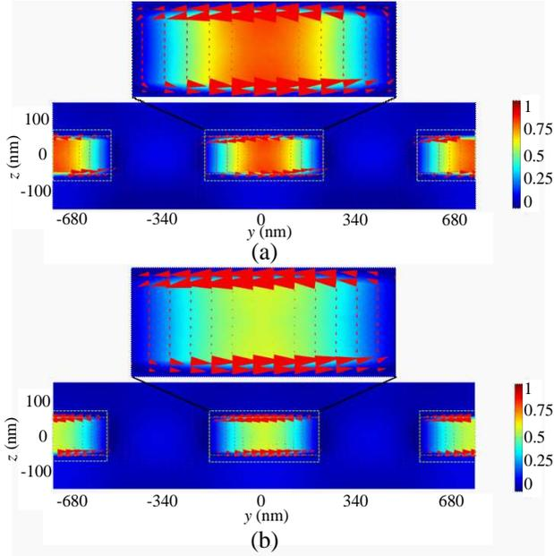
**Figure 4.** (a) A map of the normalized magnetic field intensity distribution at 1658 nm resonance wavelength for a cross section along the  $\beta$  plane ( $z$ - $x$  plane) in the ENA, a zoom in picture has been presented in the top inset. (b) A map of the normalized magnetic field intensity distribution at 1640 nm resonance wavelength for a cross section along the  $\beta$  plane ( $z$ - $x$  plane) in the CNA a zoom in picture has been presented in the top inset.
