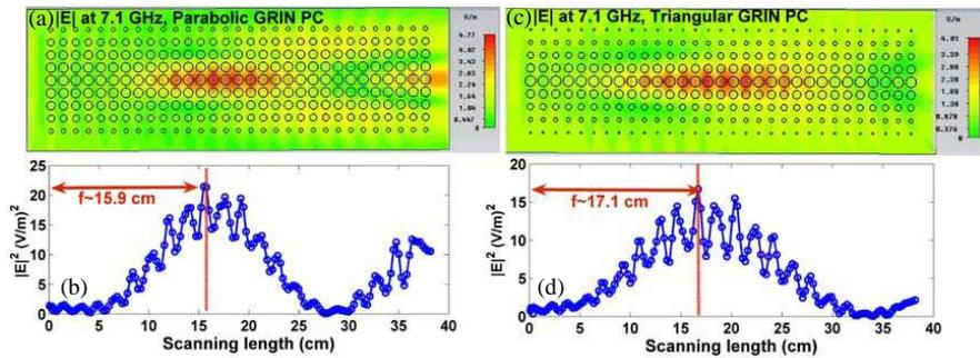
**Figure 2.** (a) and (b) show the focusing and the corresponding scanning plot of the parabolic GRIN medium. (c) and (d) show the focusing and the scanning plot for the triangular index GRIN medium. Both use a gradient coefficient of  $\alpha = 0.1172a^{-1}$  at 7.1 GHz.
