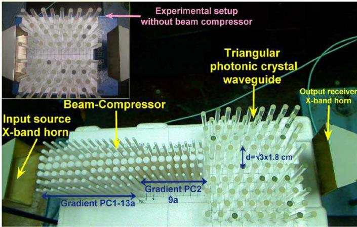
**Figure 8.** Experimental setup for an effective beam injection. The beam compressor has a length of 26.4 cm, and the PC waveguide has a length of 14.4 cm. This picture shows the X-band horn as the transmitter and receiver. Inset of the figure shows the setup for an empty PC waveguide.
