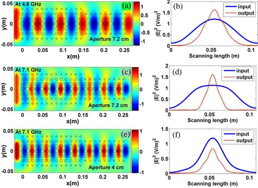
**Figure 4.** (a)  $E_z$  field map at 4.8 GHz for the finite aperture size of 7.2 cm and (b) shows the corresponding electric field intensity profiles at the input (*i/p*)/output (*o/p*) planes. (c)  $E_z$  field map at 7.1 GHz for the aperture size of 7.2 cm and (d) shows the corresponding  $|E|^2$  profiles of the *i/p* and *o/p* beams. (e)  $E_z$  field map at 7.1 GHz for the aperture size of 4 cm and (f) shows the corresponding  $|E|^2$  profiles of the *i/p* and *o/p* beams.
