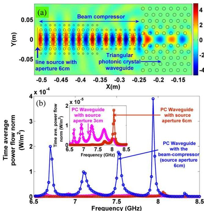
**Figure 7.** Numerical result of an effective beam injection. (a)  $E_z$  field map at 7.5 GHz shows the effective coupling provided by the beam compressor for a source aperture of 6 cm. (b) Time-averaged power flow norm is plotted for the configurations of empty PC waveguide with source apertures of 6 and 3 cm (given in the inset), and the PC waveguide with the beam compressor for the source aperture of 6 cm.
