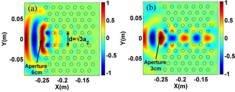
**Figure 6.** The role of source aperture for an effective-beam injection in a photonic crystal waveguide. (a)  $E_z$  field map at 7.5 GHz corresponds to the source's aperture of 6 cm. (b)  $E_z$  field map at 7.5 GHz to the source aperture of 3 cm. The PC waveguide is formed by the removal of center of row of rods in a  $14 \times 11$  layers of triangular lattice photonic crystal (defect spacing is  $d = \sqrt{3}a_2$ , where ' $a_2$ ' is the lattice constant taken to be 1.8 cm).
