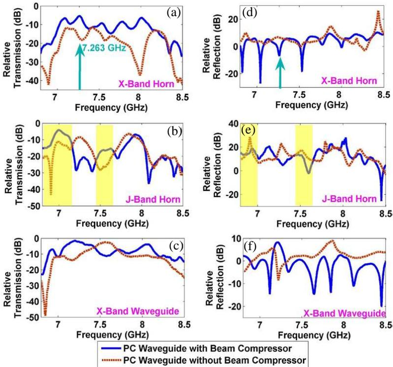
**Figure 9.** (a)–(c) shows the relative transmission parameter and (d)–(f) shows the relative reflective parameter for the PC waveguide with (blue solid line) and without (red dashed line) the beam compressor for the apertures of X-band horn antenna, J-band horn antenna, and X-band waveguide. The term ‘relative’ refers to the comparative transmission/reflection value between the structure and an air background.
