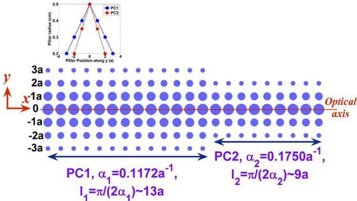
**Figure 3.** Design of beam-aperture modifier with respect to the triangular index profile. Explicit position of the pillars and its radius variation is given in the inset.
