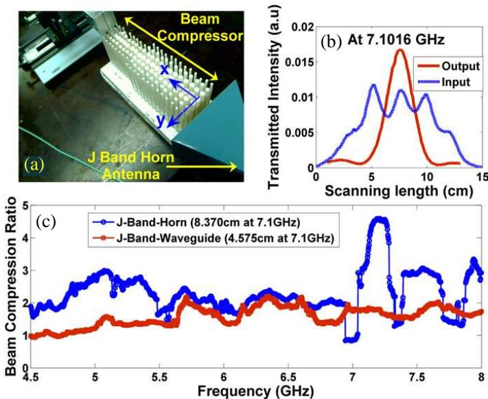
**Figure 5.** (a) Experimental setup for the beam compression studies. (b) Transmitted intensity profiles of the input and output beam scanned at 7.1016 GHz. (c) Beam compression ratio over a working frequency range of 4.5 to 8 GHz. Blue circled line corresponds to a larger beam aperture (J-band horn) and the red squared line corresponds to a smaller beam aperture (J-band waveguide).
