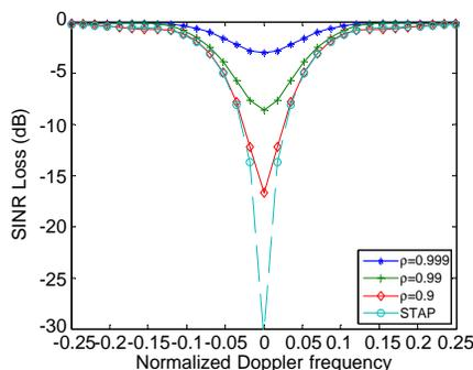
**Figure 9.** SINR loss versus target Doppler frequency in the case of different clutter polarization degree for PST-JDP method,  $\rho = 0.999$ ,  $\rho = 0.99$ ,  $\rho = 0.9$ , and SINR loss versus target Doppler frequency for STAP method.
