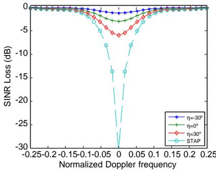
**Figure 13.** SINR loss versus target Doppler frequency in the case of different target phase difference for PST-JDP method,  $\eta = -30^\circ, \eta = 0^\circ, \eta = 30^\circ$ , clutter is completely polarized.
