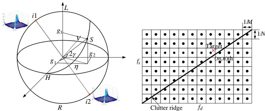
**Figure 3.** Polarization position on Poincare sphere. **Figure 4.** Resolution grids.
