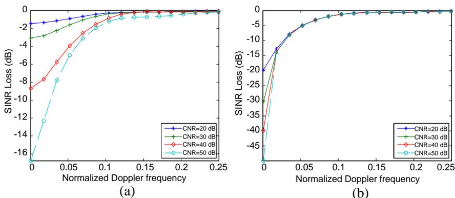
**Figure 11.** (a) SINR loss versus target normalized Doppler frequency in the case of different CNR for PST-JDP method. (b) SINR loss versus target normalized Doppler frequency in the case of different CNR for STAP method,  $CNR = 20$  dB, 30 dB, 40 dB, 50 dB.
