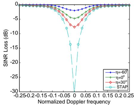
**Figure 10.** SINR loss versus target Doppler frequency in the case of different target phase difference for PST-JDP method,  $\eta = -60^\circ$ ,  $\eta = 0^\circ$ ,  $\eta = 30^\circ$ , and SINR loss versus target Doppler frequency for STAP method.
