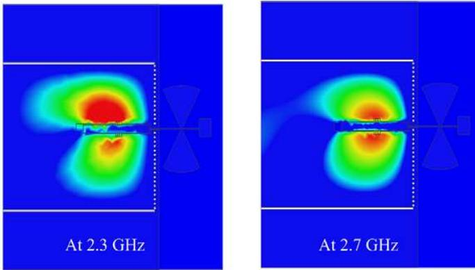
**Figure 4.**  $E$ -fields of the proposed SIW frequency-agile slot antenna.
