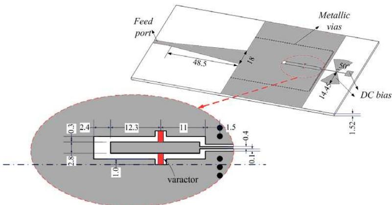
**Figure 1.** Configuration of the proposed SIW frequency-agile slot antenna. (Unit: mm).
