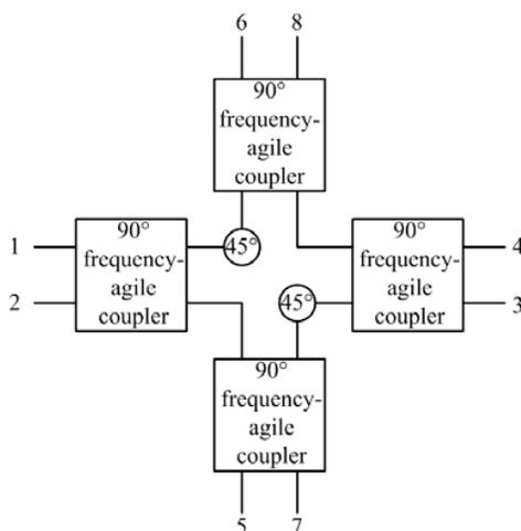
Figure 11. Configuration of the employed Butler matrix.
