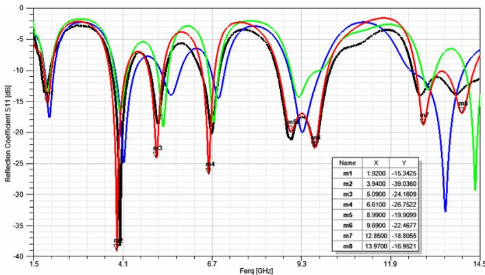
**Figure 6.** Reflection coefficient  $S_{11}$  of  $K_iS_j$  SKLB multifractal dipole (red —  $K_4S_4$  simulated, green —  $K_0S_4$ , blue —  $K_4S_0$ , black —  $K_4S_4$  measured).
