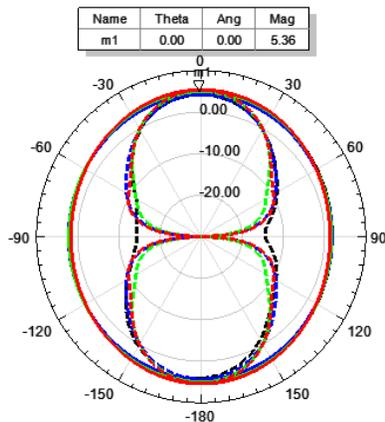
**Figure 8.** Gain patterns of  $K_iS_j$  at  $f_2$  (red —  $f_2 = 3.94$  GHz-simulated  $K_0S_4$ , black —  $f_2 = 4.027$  GHz-measured  $K_4S_4$ , green —  $f_2 = 4.04$  GHz- $K_0S_4$ , blue —  $f_2 = 4.13$  GHz- $K_4S_0$ ; solid —  $\Phi = 0^\circ$ - $XOZ$ , dash —  $\Phi = 90^\circ$ - $YOZ$ ).
