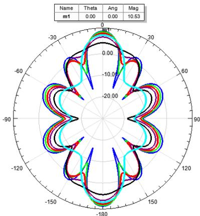
**Figure 13.**  $E$ -plane ( $\Phi = 90^\circ$ - $YOZ$ ) gain patterns of  $K_4S_4$  SKLB multifractal dipole at  $f_5 = 9.335$  GHz with sweep of  $\delta_3$  ( $G_{\max} = 10.53$  dBi; blue —  $\delta_4 = 0.6$ , green —  $\delta_4 = 0.8$ , red —  $\delta_4 = 1.0$ , purple —  $\delta_4 = 1.2$ , black —  $\delta_4 = 1.4$ , cyan —  $\delta_4 = 1.6$ )
