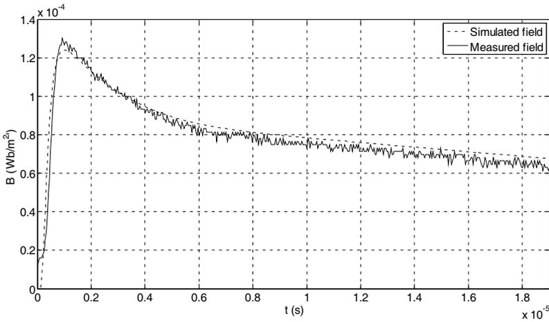
**Figure 6.** Comparison between the simulated magnetic flux density and the corresponding measured field at  $r = 30 \text{ m}$  when the MTLT current model is applied to proposed method.
