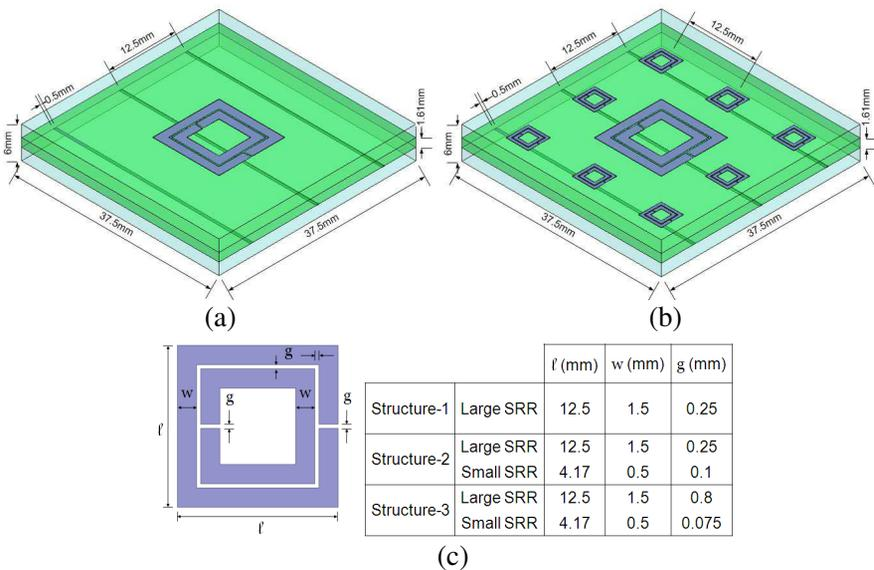
**Figure 1.** (a) Structure-1. (b) Structure-2. (c) SRR dimensions.
