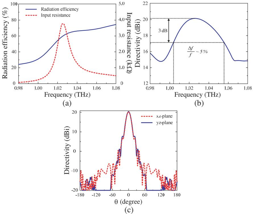
**Figure 8.** Simulated results of the optimized antenna (a) input resistance and radiation efficiency, (b) directivity, and (c) radiation patterns at the resonance frequency of 1.03 THz.
