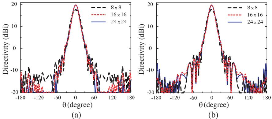
**Figure 5.** Radiation patterns in (a) the  $x$ - $z$  plane and (b) the  $y$ - $z$  plane of the antenna with different numbers of holes in the array where  $A = 2000 \mu\text{m}$ .
