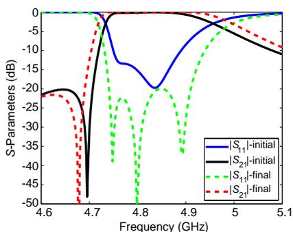
**Figure 2.** Scattering parameters for the initial dimensions ( $x_{str}$  in Table 1) and final dimensions ( $x_{opt}$  in Table 1) of a 3-pole generalized Chebyshev in-line SIW filter with one transmission zero.
