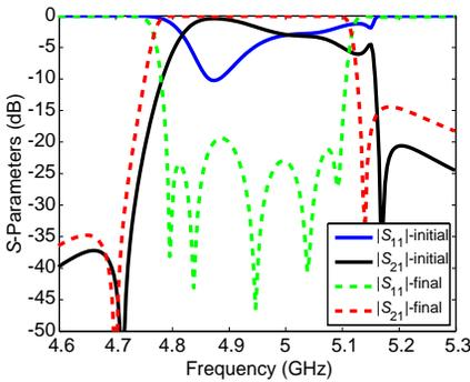
**Figure 7.** Scattering parameters for the initial dimensions ( $x_{str}$  in Table 2) and final dimensions ( $x_{opt}$  in Table 2) of a 5-pole generalized Chebyshev in-line SIW filter with two transmission zeros.
