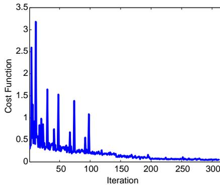
**Figure 12.** Convergence of the optimization routine for a 5-pole in-line SIW filter with two transmission zeros using a quasi-Newton algorithm with cost function defined using values of scattering parameters at position of the reflection and transmission zeros ([32]).
