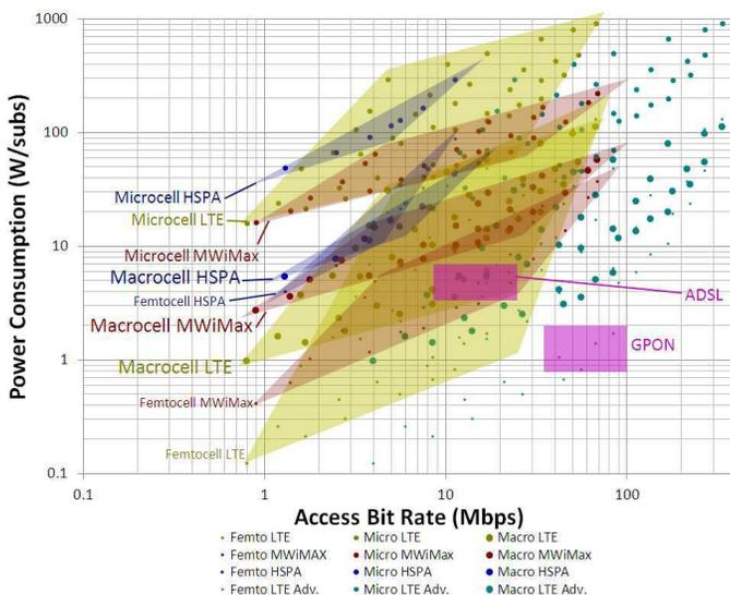
**Figure 2.** Power consumption per subscriber versus bit rate for mobile WiMAX (black x), LTE (black circle), HSPA (grey +), and LTE Advanced (grey diamond) and femto — (•), micro — (●) and macrocells — (●).
