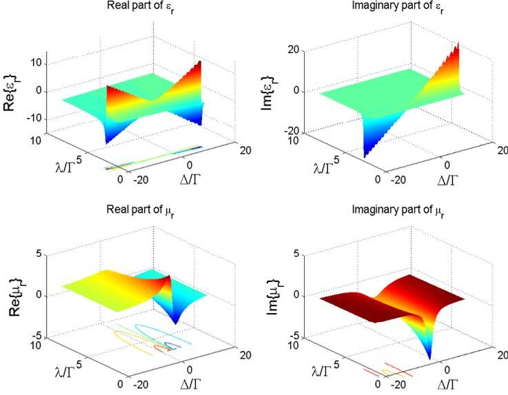
**Figure 4.** The relative permittivity and permeability versus the normalized frequency detuning  $\Delta/\Gamma$  and the normalized pumping rate  $\lambda/\Gamma$ . There are some frequency bands, in which both the permittivity and the permeability have negative real parts. The imaginary parts of the permittivity and the permeability can also be negative in these bands.
