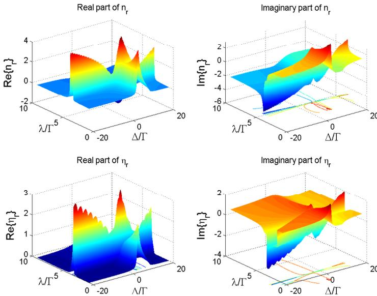
**Figure 5.** The relative refractive index  $n_r$  and the relative impedance  $\eta_r$  versus the normalized frequency detuning  $\Delta/\Gamma$  and the normalized pumping rate  $\lambda/\Gamma$ . There are some frequency bands, in which the refractive index has its negative real part, and the imaginary part can also be negative in these bands (high-gain optical amplification).
