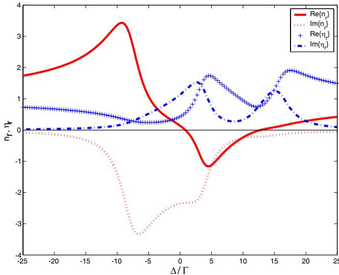
**Figure 3.** The dispersion characteristics of the real and imaginary parts of the relative refractive index  $n_r$  and the relative impedance  $\eta_r$ . There are some bands, where both the real and the imaginary parts of the refractive index are negative.
