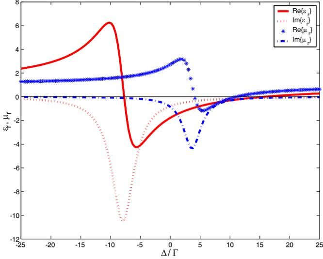
**Figure 2.** The dispersion characteristics of the real and imaginary parts of the relative electric permittivity  $\varepsilon_r$  and the relative magnetic permeability  $\mu_r$ . The simultaneously negative permittivity and permeability emerge in the frequency detuning range  $[4.5\Gamma, 11.0\Gamma]$ , and thus the atomic vapor becomes a gain LHM, since the imaginary parts of both  $\varepsilon_r$  and  $\mu_r$  in this frequency band are negative.
