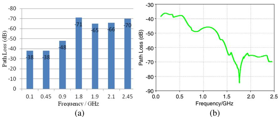
**Figure 6.** Path loss for the source position at B (lower esophagus): (a) with exact tissue property; (b) with the tissue property considered in Table 2.
