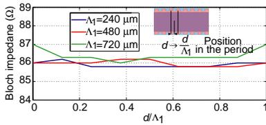
**Figure 6.** Calculated even mode Bloch impedance of the first section fixing the beginning of the unit cell in several positions of the period ( $d/\Lambda_1$ ). ( $D_1 = 280 \mu\text{m}$ ,  $G_1 = 1.72 \text{ mm}$  and  $\eta = 0.5$ ).
