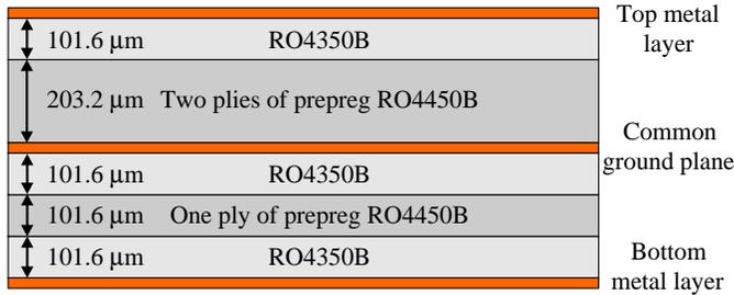
**Figure 9.** Symmetrical multilayer stack made with RO4350B substrate.
