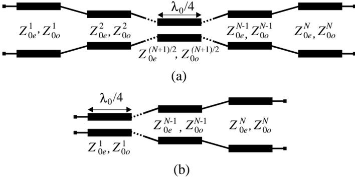
**Figure 1.** Multisection directional coupler circuit diagram. (a) Symmetric configuration. (b) Asymmetric configuration.
