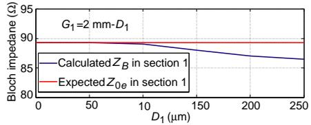
**Figure 7.** Calculated even mode Bloch impedance for the first section of the directional coupler as a function of  $D_1$  with  $\eta = 0.5$ ,  $\Lambda_1 = 240 \mu\text{m}$  and keeping the equivalent slot width ( $S_{eq1}$ ) constant to 2 mm (i.e., setting  $G_1 = 2 \text{ mm} - D_1$ ).
