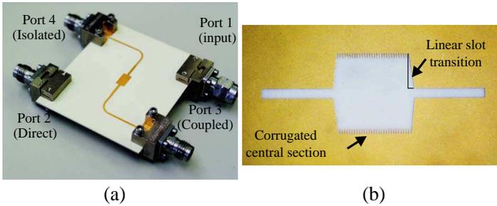
**Figure 13.** (a) Photograph of the three-section quadrature hybrid. (b) Photograph of the slot showing the corrugations, used to equalize mode phase velocities, and the linear slot transition, used to compensate discontinuity parasitics.
