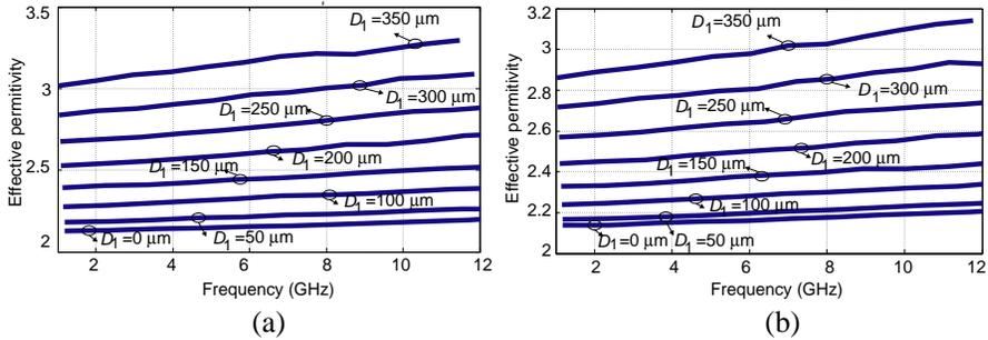
**Figure 8.** Even mode effective permittivities of the first section ( $\varepsilon_{eff_e}^1$ ) for different teeth depths ( $D_1$ ) assuming  $\eta = 0.5$  and  $G_1 = 2 \text{ mm} - D_1$  (5). (a)  $\Lambda_1 = 240 \mu\text{m}$ . (b)  $\Lambda_1 = 480 \mu\text{m}$ .
