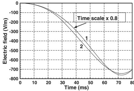
**Figure 4.** Leader field at 5 km. Curve 1 is due to a straight channel with height 10 km. The time scale of the field has been multiplied by 0.8 for the ease of comparison. Curve 2 is due to a channel with 5 km vertical length and 3 km horizontal upper part inclined away from the observer.
