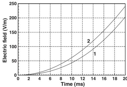
**Figure 3.** Leader field at 5 km. Curve 1 is due to a straight channel with height 2 km and Curve 2 is leader field of a channel with 5 km vertical length and 3 km horizontal upper part inclined towards the observer.
