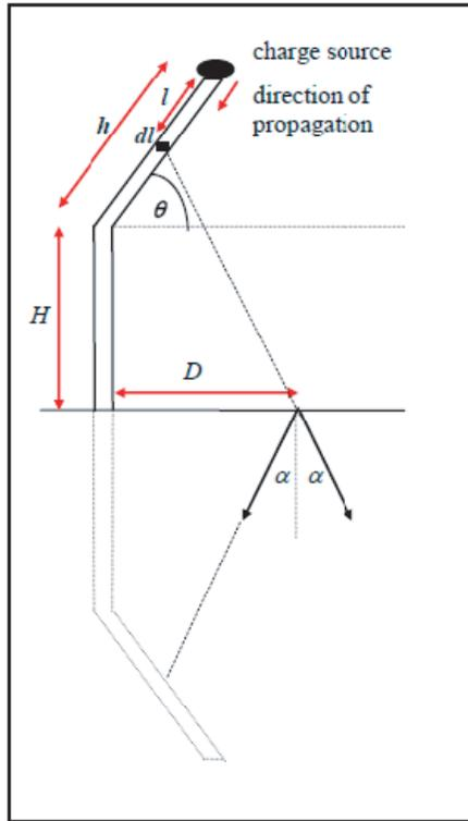
**Figure 1.** The geometry of the channel and its image that contributes to the electric field at ground at a distance  $D$  from the channel base. The arrows at distance  $D$  shows the direction of field components due to an infinitesimal channel length  $dl$  at height  $H + (h-l) \sin \theta$ . At time  $t$ ,  $l = vt$  where  $v$  is the leader speed.
