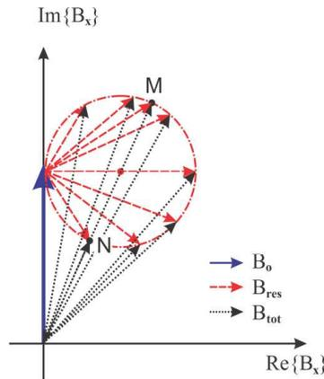
**Figure 2.** Response of an RLC meta-atom: Phasors of the source (blue, continuous), resonator (red, dashed), and total (black, dotted) magnetic flux density. The circle is the trace of meta-atom magnetic flux density for frequencies from 0 to infinity [12]. M and N points show the points at which the total magnetic flux density is maximum and minimum respectively.
