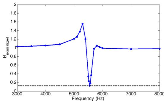
**Figure 11.** Frequency response of a metamaterial built by meta-atoms with two coils and lattice phase equalizer.  $B_{\text{normalized}}$  is the magnetic flux density normalized to the source magnetic flux density. The suppression effect of the lattice phase equalizer on the enhancement below resonance is seen clearly.
