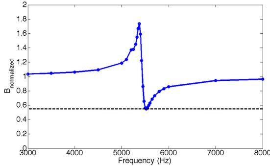
**Figure 7.** Frequency response of a metamaterial built by RLC resonators.  $B_{\text{normalized}}$  is the magnetic flux density normalized to the source magnetic flux density. First, it is seen that metamaterial shows an enhancement reaching up to 73%, and when the frequency increases it starts to shield and maximum shielding is 45% at the point where the frequency response was measured.
