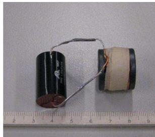
**Figure 1.** A meta-atom at low frequencies, composed of a capacitor (1  $\mu\text{F}$ ) and a coil (1 mH).
