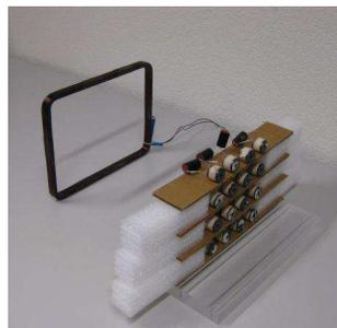
**Figure 6.** An illustration of the experimental setup for a metamaterial built by RLC meta-atoms. The large coil is used as magnetic field source and the metamaterial is a  $4 \times 4$  array of coil and capacitor pairs.
