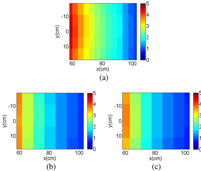
**Figure 8.** The spatial distribution of magnetic flux density without and with metamaterial. The color shows the magnetic flux density in  $\mu\text{T}$ . The source coil is at  $(x = 0, y = 0)$ . (a) The magnetic flux density of the source coil. (b) The magnetic flux density with the metamaterial located at  $x = 14$  cm. (c) The magnetic flux density with the metamaterial located at  $x = 38$  cm.
