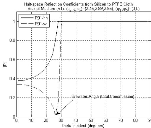
**Figure 6.** Co-polarized reflection coefficients from Silicon-PTFE cloth boundary.
