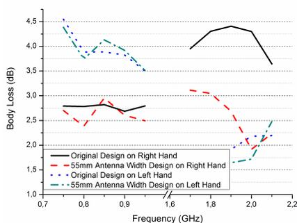
**Figure 11.** The body loss in the data mode.
