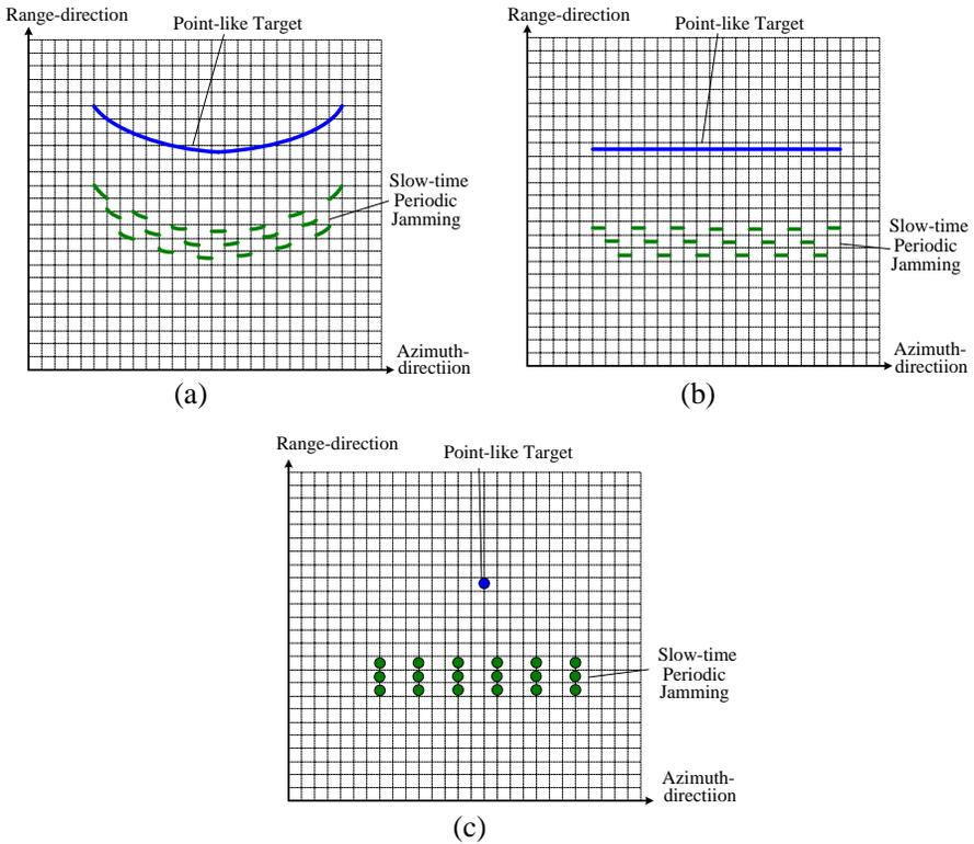
**Figure A2.** SAR imaging results of DRFP with periodic modulations in both directions. (a) SAR imaging after pulse compression in range-direction. (b) SAR imaging after RCMC. (c) SAR imaging after two-dimensional pulse compressions.
