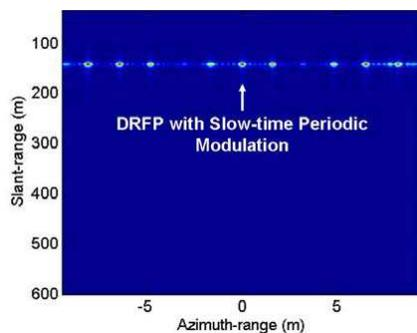
**Figure 3.** DRFP with slow-time periodic modulation. (Horizontal: Azimuth-direction; Vertical: Range-direction).
