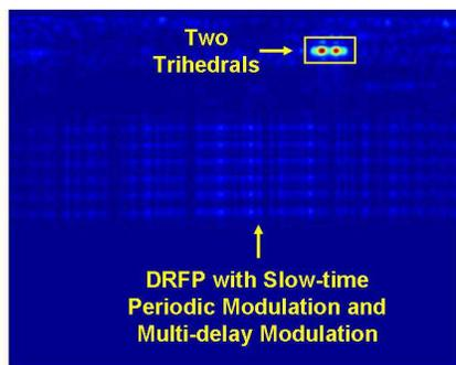
**Figure 11.** SAR imaging result of DRFP with slow-time periodic modulation and multi-delay modulation.
