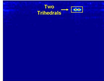
**Figure 9.** SAR imaging results without jamming.
