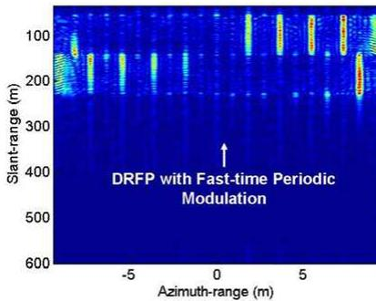
**Figure 6.** DRFP with fast-time periodic modulation. (Horizontal: Azimuth-direction; Vertical: Range-direction).
