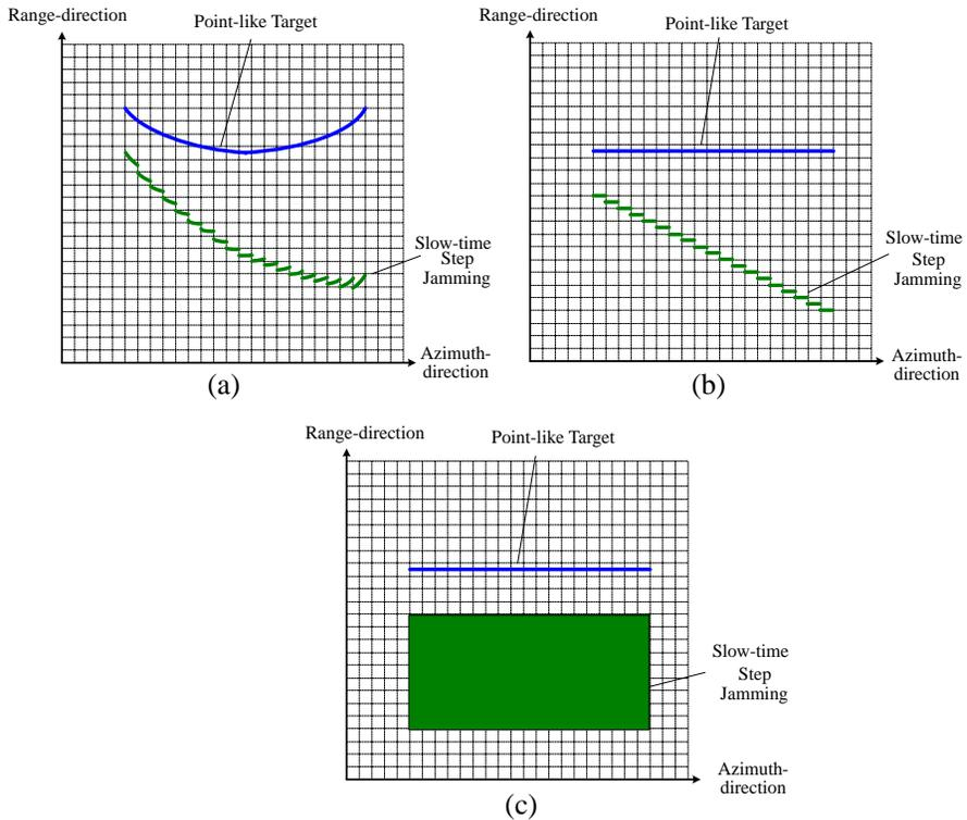
**Figure A1.** SAR imaging results of DRFP with stepped modulations in both directions. (a) SAR imaging after pulse compression in range-direction. (b) SAR imaging after RCMC. (c) SAR imaging after two-dimensional pulse compressions.
