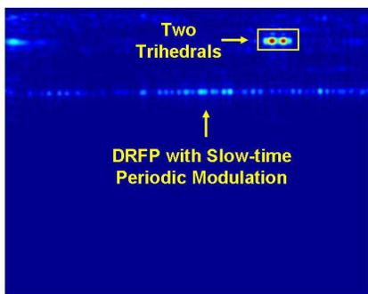
**Figure 10.** SAR imaging result of DRFP with slow-time periodic modulation.
