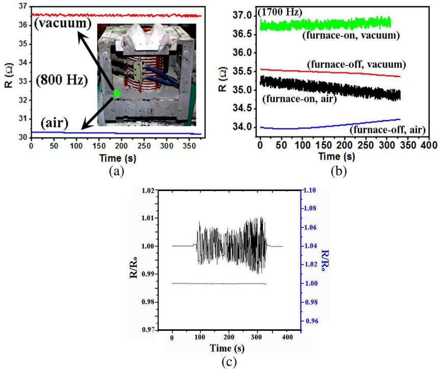
**Figure 7.** The real time sensing profiles obtained from a high-frequency inductive furnace at (a) 800 Hz, and at (b) 1700 Hz. Insert: side-view of inductive furnace and green spot denotes the measuring point. (c) Sensing with (blue) and without (dark) foil shielding.
