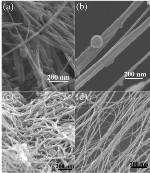
**Figure 8.** SEM images of (a) arc-made MWCNTs before and (b) after a series of physicochemical treatments, and (c) arc-made SWCNTs before and (d) after a series of physicochemical treatments.
