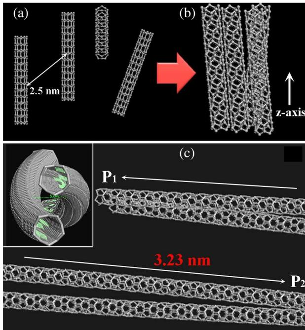
**Figure 10.** Bundling of (a)–(b) separated tubes, and (c) a full pitch of helicity ( $P_1 \rightarrow P_2$ ). Insert: side-view of twisted tubes.
