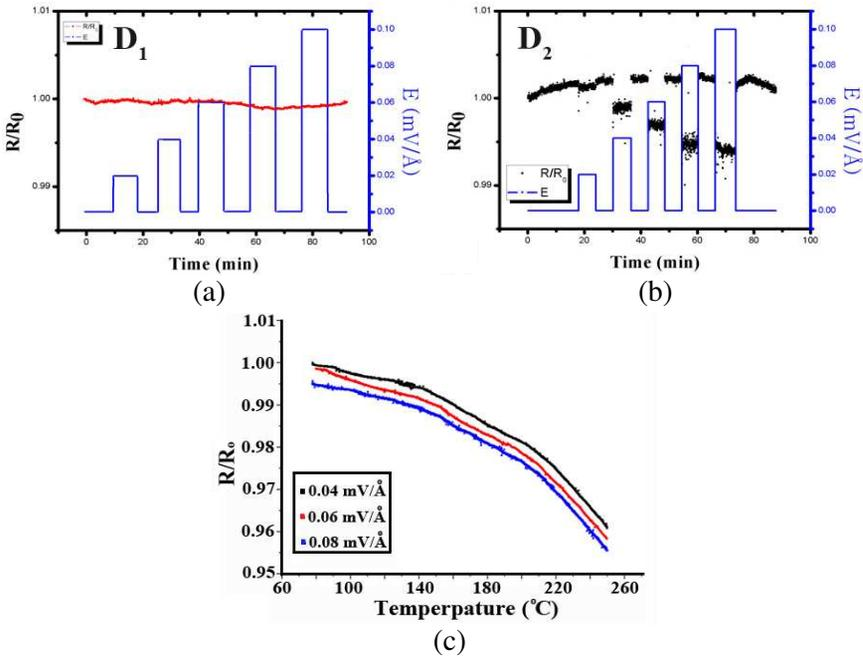
**Figure 5.** The  $R/R_o$ - $E$  plots of (a)  $D_1$ , (b)  $D_2$ , and (c)  $R/R_o$ - $T$  plots of  $D_2$ .
