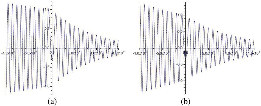
**Figure 4.** Numerical results (blue dash line) vs analytical results (black solid line) for electric field  $E(x)$  as a function of  $x$ , with  $E_0 = 1$ ,  $k = 2\pi/(10^{-6} \text{ m})$ ,  $\rho = 1/(10^{-6} \text{ m})$ ,  $\kappa\beta = 2\pi/(10^{-4} \text{ m})$  as well as (a)  $\alpha = 0.75\kappa\beta$  and (b)  $\alpha = 0.50\kappa\beta$ .
