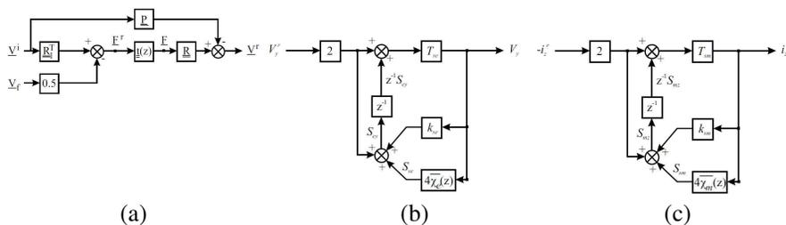
**Figure 3.** (a) Signal flow diagram of the general algorithm of TLM method based on Z-transform [36]. (b) Dispersive TLM Z-transform model for metamaterials — calculation of  $E_y$  in the time-domain. (c) Dispersive TLM Z-transform model for metamaterials — calculation of  $H_z$  in the time-domain.
