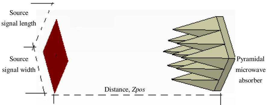
**Figure 4.** Simulation setup for CST's microwave studio simulation.
