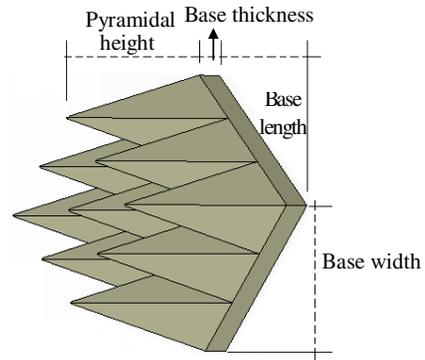
**Figure 3.** SCB pyramidal microwave absorber designed in CST's microwave studio.
