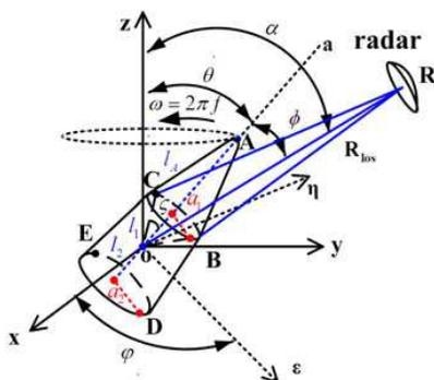
**Figure 1.** Geometry of radar and BT with precession.
