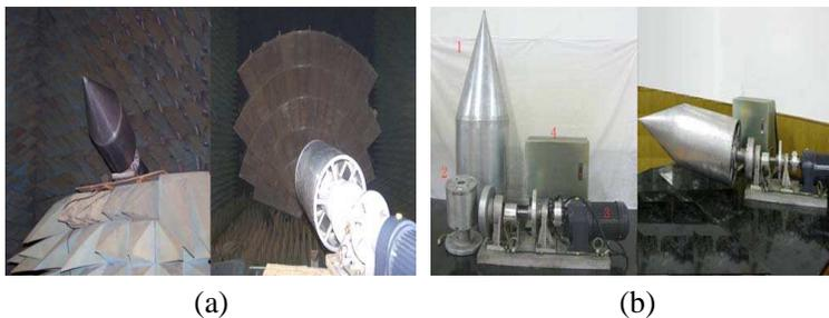
**Figure 3.** Measurement of the BT model in the microwave anechoic chamber. (a) The measurement setting. (b) Precession model of BT.
