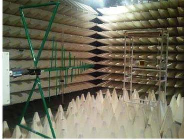
**Figure 9.** Antenna under test (AUT) in chamber.
