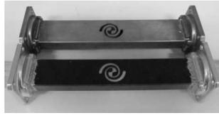
**Figure 6.** Spiral SWA manufactured from copper and brass flanges (upper image), and CFRP and aluminium flanges (lower image).
