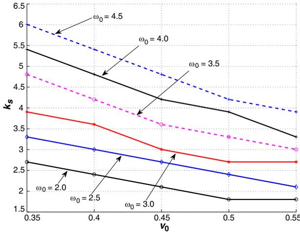
**Figure 3.** The dependence of the spectral peak position (wavenumber  $k_s$ ) of the field  $E_x(x, t)$  on the particle velocity  $v_0$  for different  $\omega_0$  at  $t \sim 190$  in dispersiveless case.
