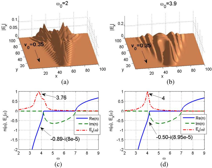
**Figure 5.** The same as in Fig. 4 but for velocity  $v_0 = 0.35$ . (a) Field  $E_x$  for  $\omega_0 = 2$  that generates the plasmon-polaritons excitation (PPE) at the peak frequency  $\omega_C = 3.76$  where  $\text{Re}(n) = -0.89$  (c); (b) field  $E_x$  for  $\omega_0 = 3.9$  that generate PPE at the peak frequency  $\omega_C = 4$  where  $\text{Re}(n) = -0.50$ .
