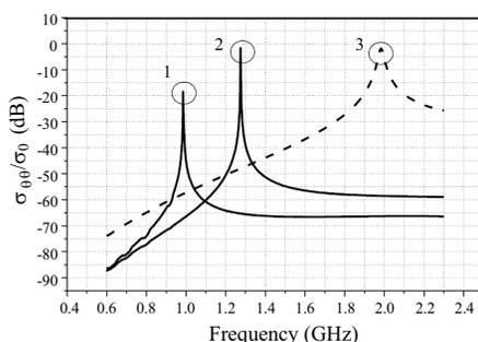
**Figure 2.** CMA radar cross section  $\sigma_{\theta\theta}/\sigma_0$  and resonant frequencies  $f$  for different-shape patches: 1 — slotted strip-frame patch,  $f_1 = 0.985$  GHz, 2 — pair of coupled slotted strip-frame patches,  $f_2 = 1.275$  GHz, and 3 — rectangular cylindrical patch,  $f_3 = 1.9825$  GHz.
