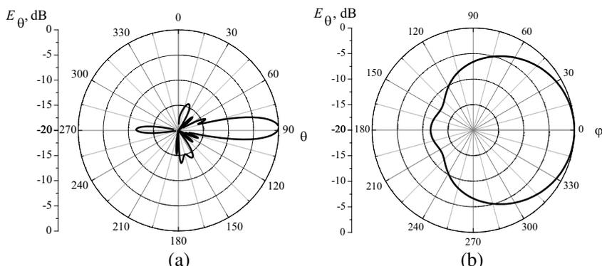
**Figure 9.** The CMAA radiation patterns at resonant frequency  $f = 1.35$  GHz: the  $E_{\theta}$ -component versus  $\theta$  with (a)  $\varphi = 0^{\circ}$  and versus  $\varphi$  with (b)  $\theta = 90^{\circ}$ .
