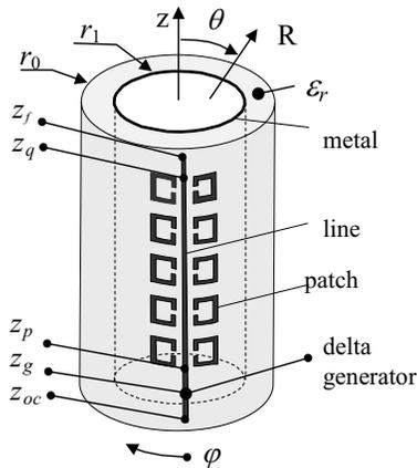
**Figure 6.** The radiating structure — the CMAA of 10 patches.
