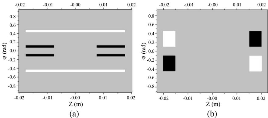
**Figure 4.** Phase distributions of the (a)  $z$ - and (b)  $\varphi$ -components of the surface current density on the pair of coupled slotted strip-frame patches.
