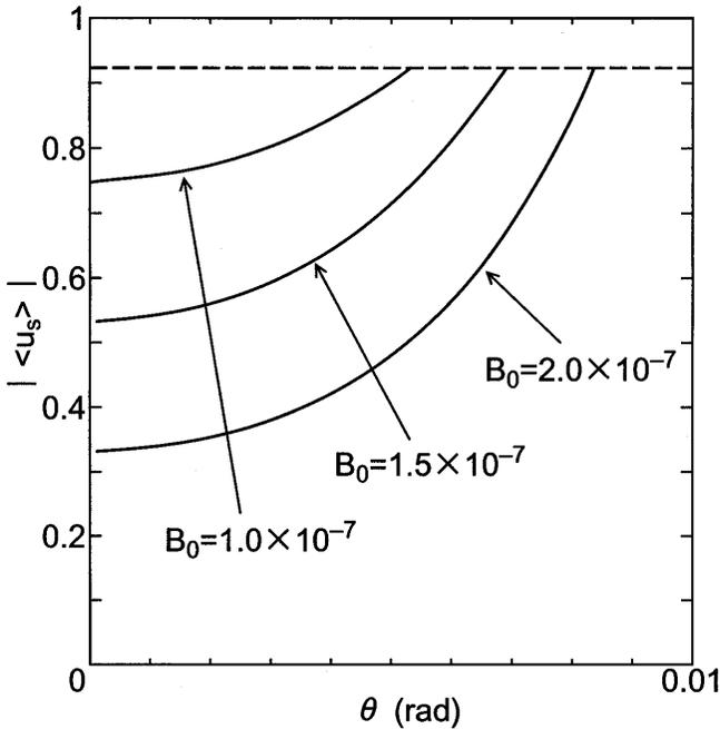
Figure 9. Bistatic scattering characteristics of the coherent wave under the condition of  $B_0 l_0$  constant, where the broken line shows that the effect of double passing is not included in  $|\langle u_s \rangle|$ .
