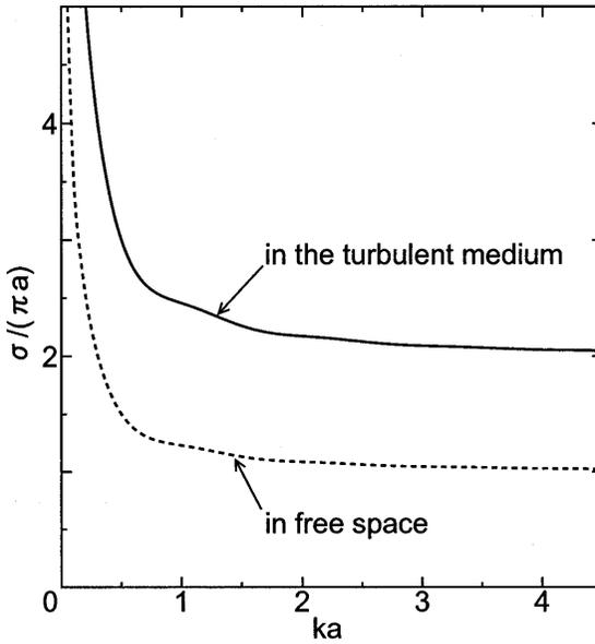
Figure 11. The average backscattering cross-section in the case of E-wave incidence, where the coherence length of the incident wave is shown in Figure 10.
