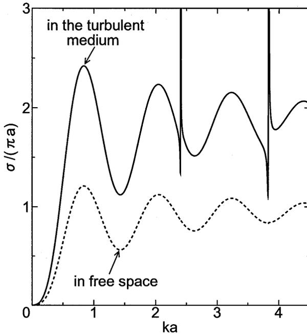
Figure 12. The average backscattering cross-section in the case of H-wave incidence, where the coherence length of the incident wave is shown in Figure 10.
