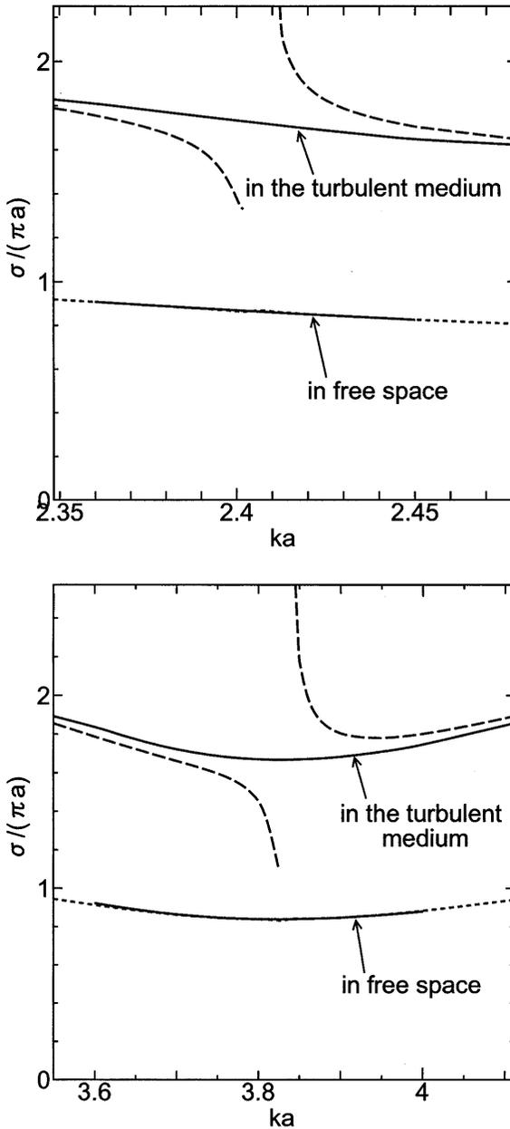
Figure 15. The average backscattering cross-sections about the internal resonance frequencies in the case of H-wave incidence. (a) In the neighborhood of the first zero point of  $J_0(ka_0)$  :  $ka_0 = 2.40482 \dots$  (b) In the neighborhood of the second zero point of  $J_1(ka_0)$  :  $ka_0 = 3.83171 \dots$ .
