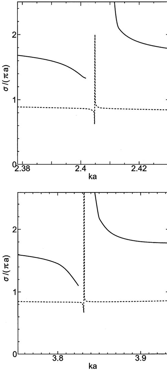
Figure 13. Enlargement of Fig. 12 about the internal resonance frequencies of the cylinder. (a) In the neighborhood of the first zero point of  $J_0(ka_0)$ :  $ka_0 = 2.40482 \dots$  (b) In the neighborhood of the second zero point of  $J_1(ka_0)$ :  $ka_0 = 3.83171 \dots$ .
