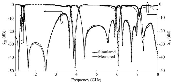
**Figure 10.** The responses of the quad-band filter.
