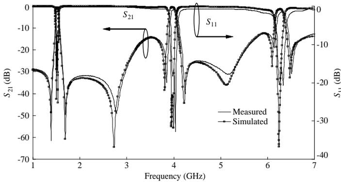
**Figure 7.** The responses of the tri-band filter.
