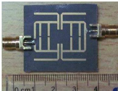
**Figure 6.** The photograph of tri-band filter.
