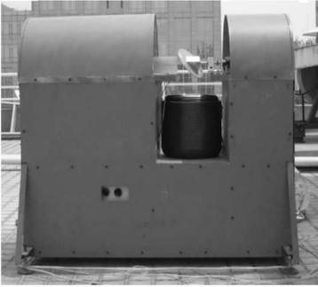
**Figure 1.** The K-band ground-based hyperspectral microwave radiometer (BHU-K80) with 80 spectral channels.
