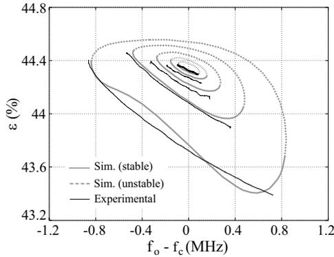
**Figure 13.** Measured efficiency of the synchronized solutions. The represented solutions have been obtained by changing the reference signal power  $P_r$  between  $-40$  and  $-20$  dBm in 5 dB steps.
