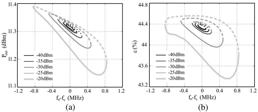
**Figure 6.** (a) Synchronized solutions in terms of the output power  $P_o$ , for different values of  $P_r$ . (b) Efficiency on the synchronized solutions. Continuous line: stable solutions. Dashed line: unstable solutions.
