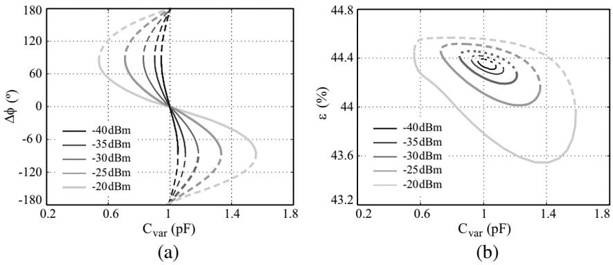
**Figure 9.** (a) Phase shifter synchronized solutions expressed in terms of the output phase and  $C_{var}$ , for different values of  $P_r$ . (b) Efficiency associated with the synchronized solutions. Continuous line: Stable solutions. Dashed line: unstable solutions.
