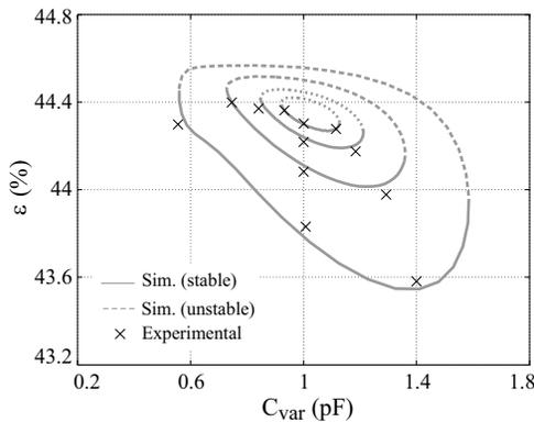
**Figure 14.** Measured efficiency of the phase shifter synchronized solutions. The represented solutions have been obtained by changing the reference signal power  $P_r$  between  $-35$  and  $-20$  dBm in 5 dB steps.
