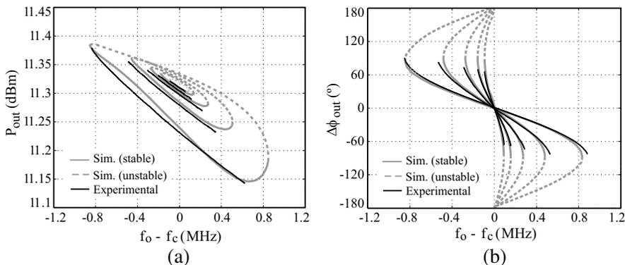
**Figure 12.** Measured synchronized solutions in terms of (a) the power  $P_o$  and (b) the phase  $\Delta\phi_{out}$  of the output signal. The represented solutions have been obtained by changing the reference signal power  $P_r$  between  $-40$  and  $-20$  dBm in 5 dB steps.
