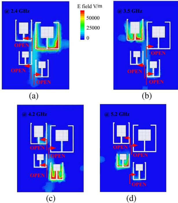
**Figure 8.** Electric field distributions for (a) the first channel @ 2.4 GHz. (b) The Second channel @ 3.5 GHz. (c) The third channel @ 4.2 GHz. (d) The fourth channel @ 5.2 GHz.
