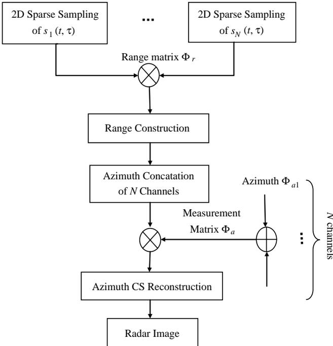
**Figure 5.** Flowchart of azimuth multichannel SAR imaging algorithm based on compressed sensing.
