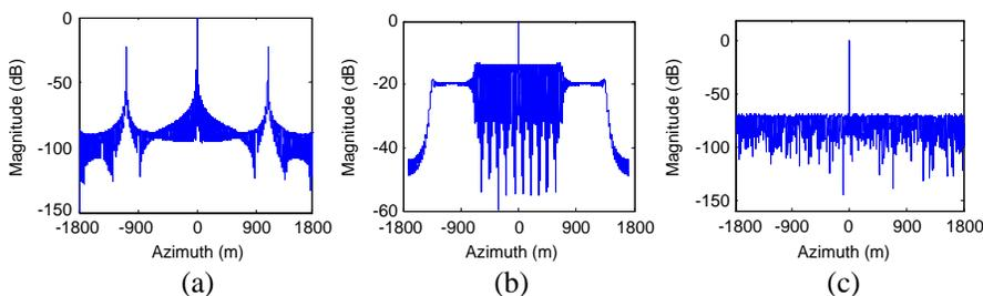
**Figure 7.** Azimuth profile of target reconstruction with different method (PRF  $\approx$  1800 Hz). (a) RD imaging with full samples before spectrum reconstruction. (b) RD imaging with full samples after spectrum reconstruction. (c) CS based recovery with 30% samples.
