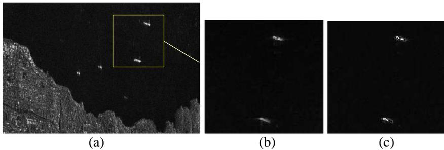
**Figure 9.** Imaging of original Radarsat-1 raw data with different methods: (a) Original radarsat-1 image with two distributed ships targets. (b) RD imaging with full samples and uniform sampling. (c) CS based recovery with 11.1% samples after nonuniform processing.
