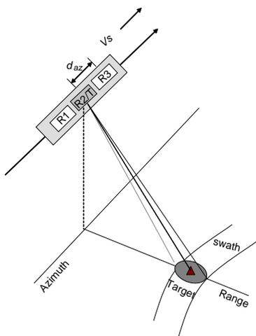
**Figure 3.** Imaging geometry model of spaceborne DPCA SAR.
