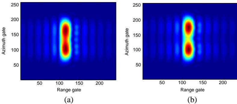
**Figure 8.** Contour of two targets  $T_1$  and  $T_2$  with both method. (a) RD imaging. (b) CS based recovery.
