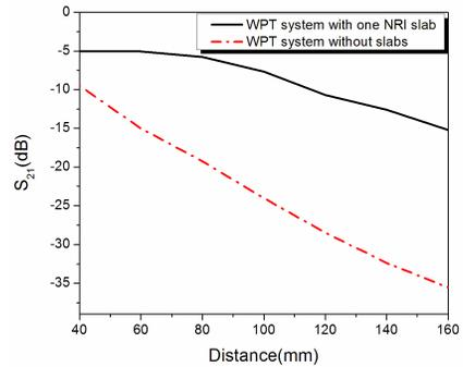
**Figure 8.** Comparison of measured  $S_{21}$  of the WPT system with and without NRI metamaterials when the distance varies.
