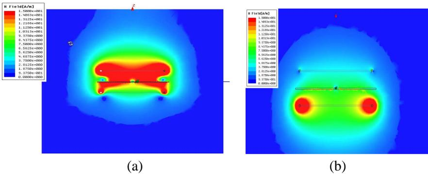
**Figure 9.** Magnetic field of the WTP system with one NRI slab. (a) Magnetic field at the negative refractive index frequency of the NRI slab, (b) magnetic field at the non-resonant frequency of the NRI slab.
