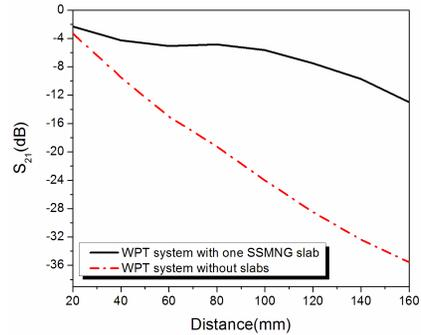
**Figure 15.** Comparison of the measured  $S_{21}$  of the WPT system with and without one SSMNG metamaterial slab when the distance varies.
