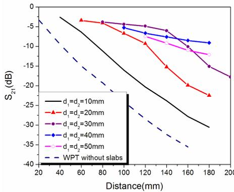
**Figure 18.** Measured  $S_{21}$  of the WPT system with two SMMNG slabs and that of WPT system without metamaterial slabs, and the distance between the copper ring and the slab varies from 10 mm to 50 mm.
