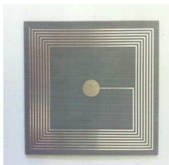
**Figure 12.** Top view of the fabricated given MNG metamaterial.
