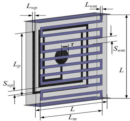
**Figure 2.** Solid view of the proposed NRI metamaterial geometry.
