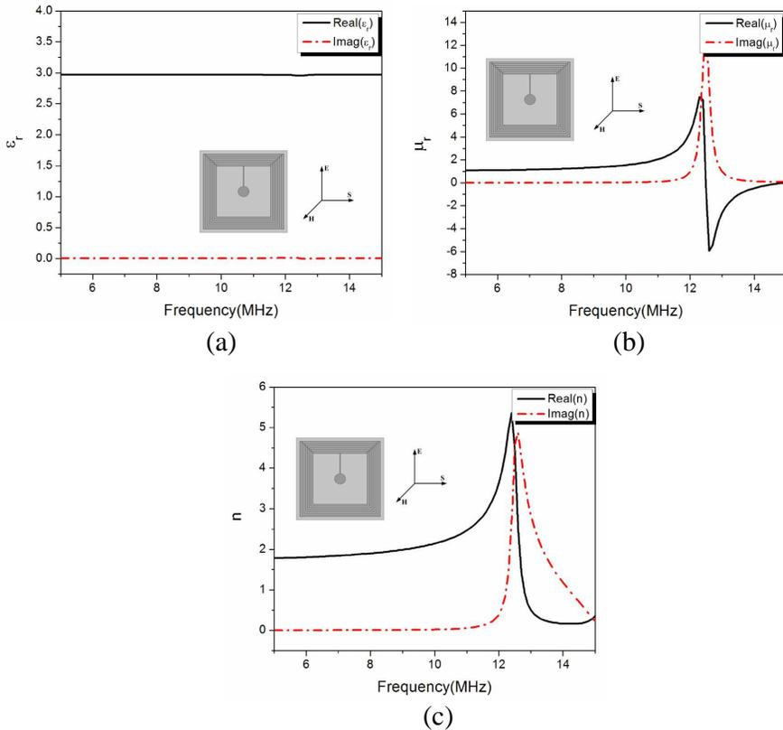
**Figure 13.** (a) Effective permittivity, (b) effective permeability, and (c) effective refractive index properties of the given MNG metamaterials.
