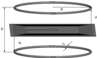
**Figure 5.** WPT system with one MNG metamaterial slab.
