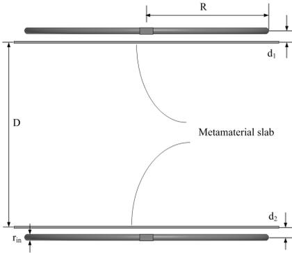
**Figure 16.** WPT system with two metamaterial slabs.
