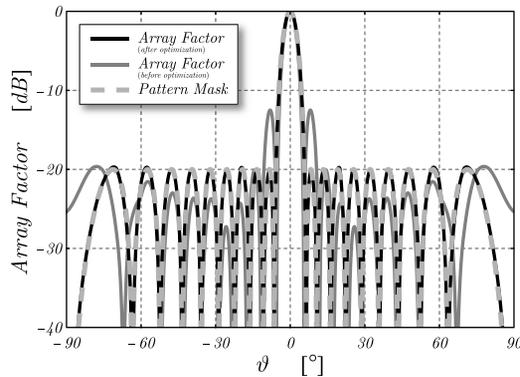
**Figure 4.** Angular behavior of the synthesized array factor useful to mimic a pencil-beam pattern mask (shown in light-gray dashed line) with side-lobe level  $SLL = -20$  dB and angular width  $\Theta = 5.5^\circ$ . As it can be noticed, the parasitic antenna coupling is responsible for a performance degradation in terms of array side-lobe levels (see dark-gray continuous line) that is compensated by means of the optimization procedure based on PSO and MNM (see black continuous line).
