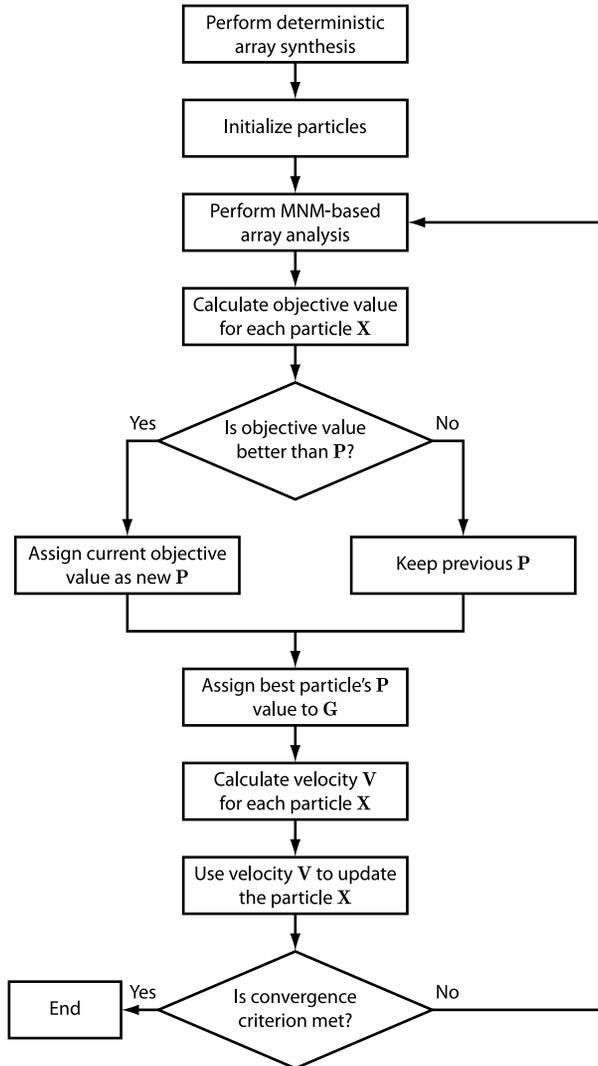
**Figure 3.** Flowchart of the hybrid deterministic/metaheuristic synthesis technique for non-uniformly spaced printed antenna arrays.
