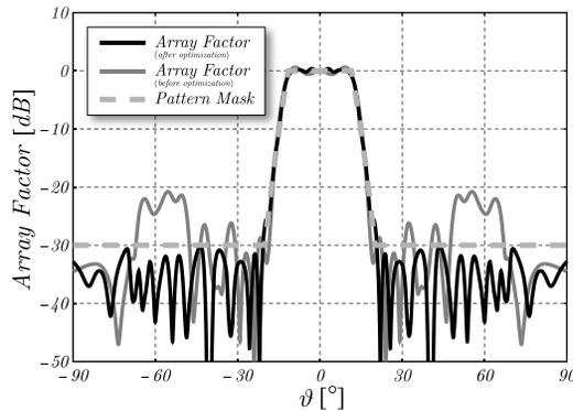
**Figure 6.** Angular behavior of a flat-top shaped-beam array factor with side-lobe level  $SLL = -30$  dB synthesized by means of  $N_a = 26$  patch antennas distributed along an aperture having size  $D_{\max} = 11.625 \lambda_0$ . The radiation pattern mask is shown in light-gray dashed line.
