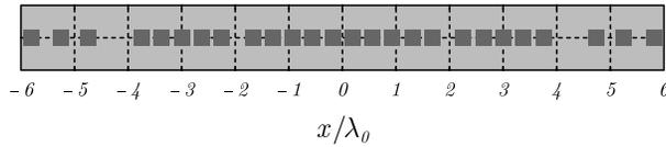
**Figure 7.** Topology of the non-uniformly spaced patch antenna array useful to mimic the shaped-beam pattern shown in Fig. 6. The minimum inter-element spacing is  $\Delta x_{\min} \simeq 0.373\lambda_0$ .
