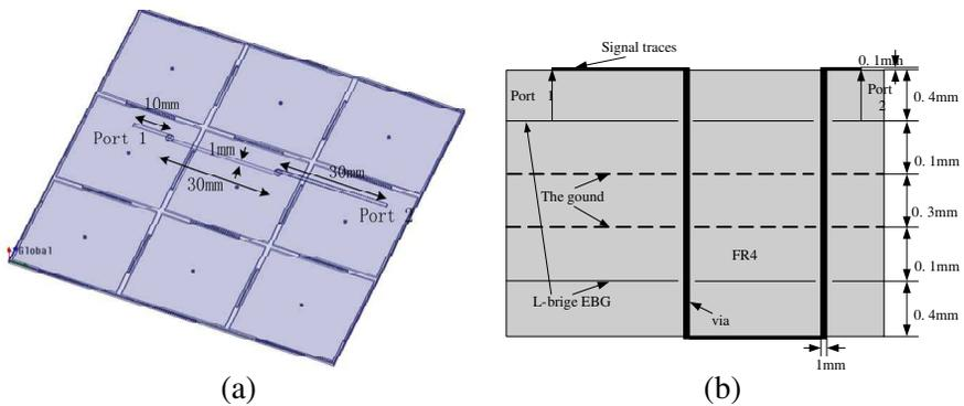
**Figure 7.** Six-layer PCB with signal layer referring to the proposed structure. (a) The three-dimensional view. (b) The side view.
