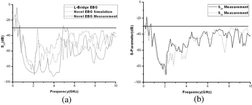
**Figure 4.** Simulated and measured insertion loss  $S$ -parameters for the novel vertical cascaded planar EBG structure. (a) The comparison of  $S_{21}$  between the L-Bridge board and the proposed design obtain by simulation and measurement. (b) The comparison of measured insertion loss including  $S_{21}$  and  $S_{31}$  for the proposed design.
