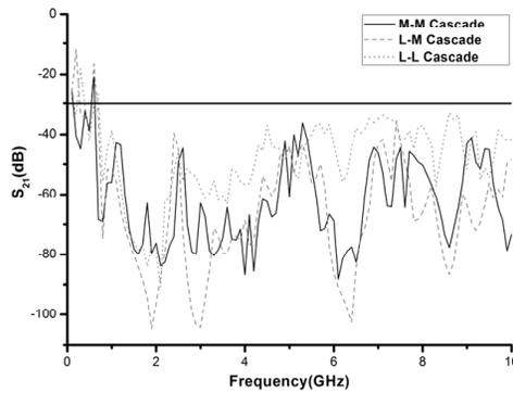
**Figure 6.** The comparison of  $S_{21}$  with the different EBG structures obtained by using vertical cascade.
