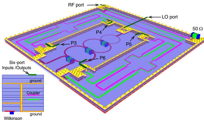
**Figure 9.** 3D view of the LTCC six-port network.
