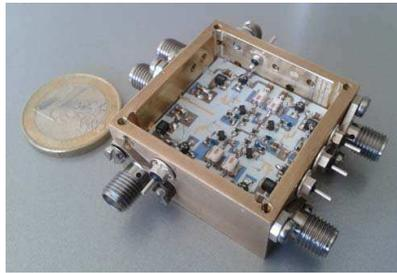
**Figure 19.** Fabricated LTCC six-port receiver prototype.
