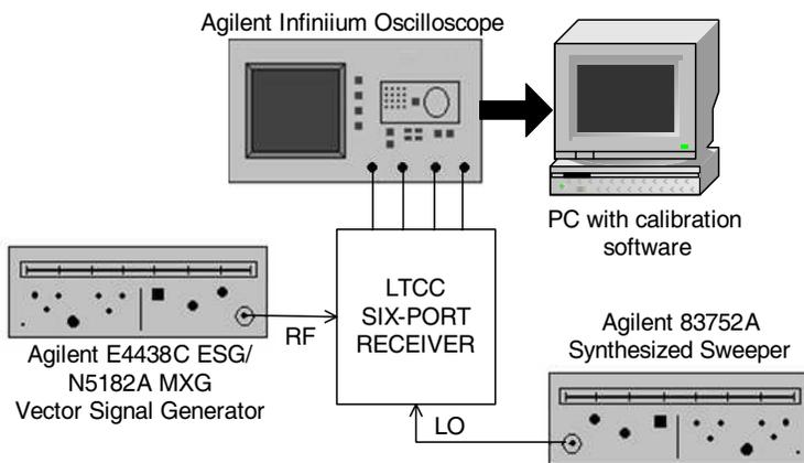
**Figure 20.** Set-up of the LTCC six-port receiver test-bench.
