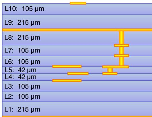
Figure 3. LTCC layer structure, DuPont-943 substrate.
