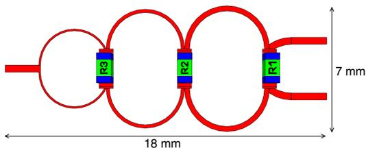
Figure 7. Layout of the Wilkinson power divider.
