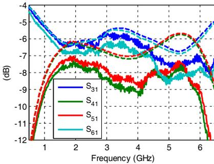
**Figure 16.** Measured (solid line) and simulated (dashed line) attenuations from the LO port.
