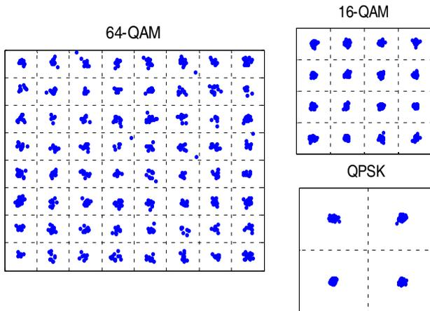
**Figure 21.** Received constellations: 15.625 Msymbol/s,  $P_{LO} = 0$  dBm,  $P_{in} = -25$  dBm.
