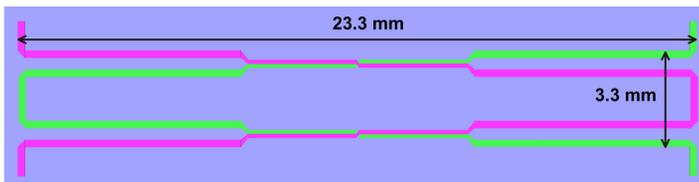
**Figure 4.** Layout of the LTCC 3-dB tandem coupler.
