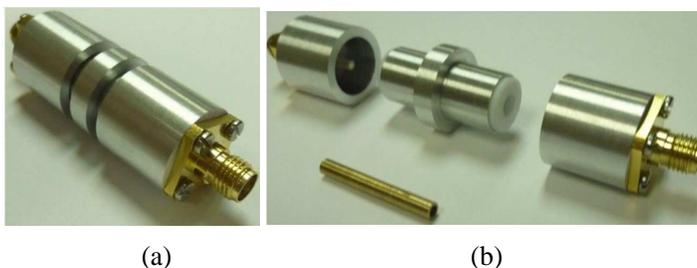
**Figure 12.** Ad-hoc connector prototype. (a) Plugged. (b) Unplugged.
