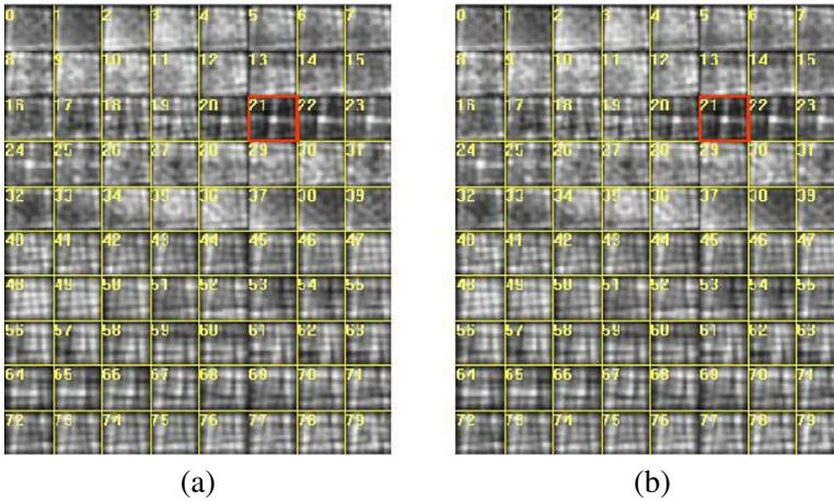
**Figure 11.** Reconstructed slices, (a) along  $z$ -axis, reconstructed from intensity measurements taken along the  $x$ - $y$  plane, (b) along  $y$ -axis, reconstructed from intensity measurements taken along the  $x$ - $z$  plane.
