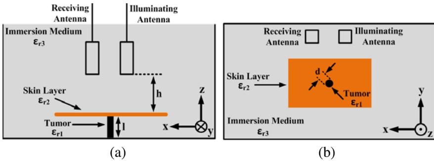
**Figure 4.** Simulated breast phantom, (a) front view,  $x$ - $z$  plane, (b) top view,  $x$ - $y$  plane ( $\epsilon_{r1} = 11.9$ ,  $\epsilon_{r2} = 4.5$ ,  $\epsilon_{r3} = 2$ ,  $l = 6$  cm,  $d = 4$  cm,  $h = 10$  cm).
