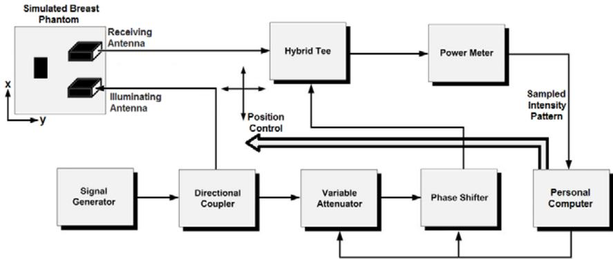
**Figure 2.** Experimental arrangement for intensity pattern formation.
