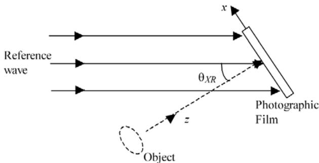
**Figure 1.** Off-axis hologram.
