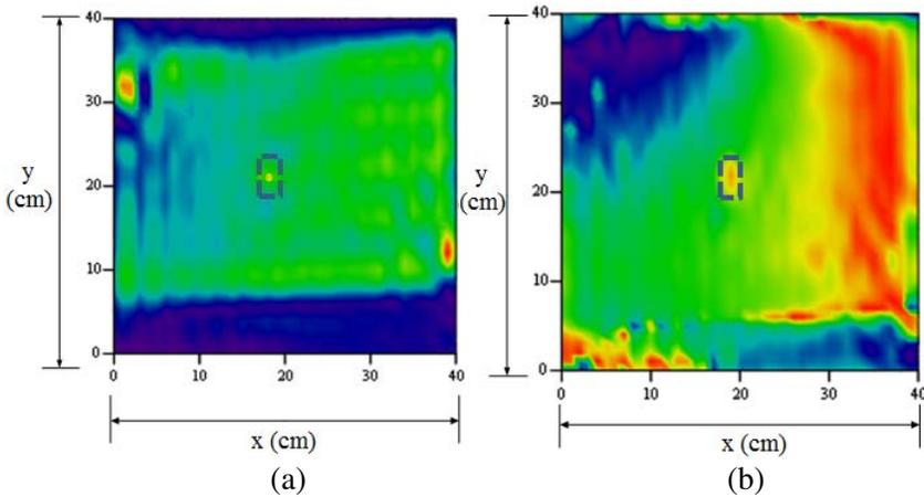
**Figure 8.** Reconstructed images of the breast phantom with the tumor highlighted, (a) magnitude image, (b) phase image.
