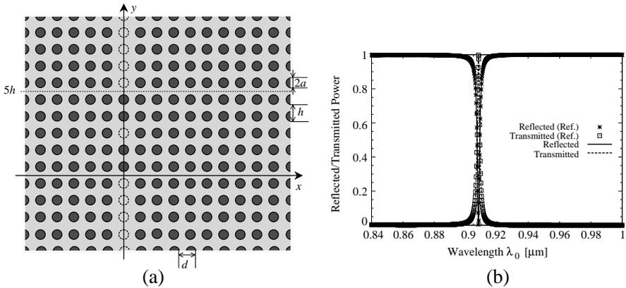
**Figure 3.** Photonic crystal waveguide filter consists of a resonance cavity weakly coupled with straight waveguides. (a) Structure under consideration. (b) Power reflection and transmission spectra.
