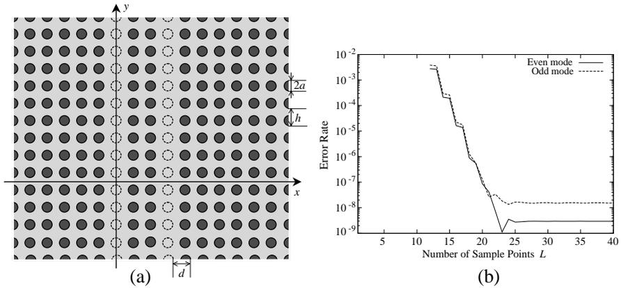
**Figure 2.** Coupled parallel photonic crystal waveguides. (a) Structure under consideration. (b) Convergence of the propagation constants.
