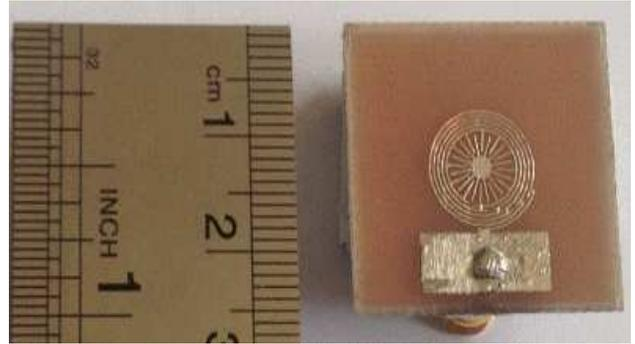
**Figure 6.** Second fabricated antenna geometry.
