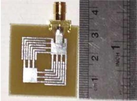
**Figure 5.** Geometrical model of the first fabricated antenna.
