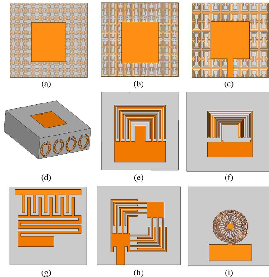
**Figure 2.** The geometry of patch antennas, (a) on fractal ground, (b) on SRR rings, (c) on dumbbell SRR rings, (d) SRR resonators, (e) Bent Interdigital capacitance, (f) with meandered load, (g) meandered Patch with Interdigital capacitance, (h) dual bent Interdigital, (i) Spiral CRLH structure.
