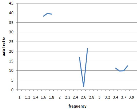
**Figure 9.** Measured axial ratio of presented antenna.
