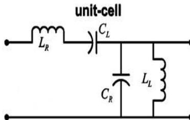
**Figure 1.** Equivalent circuit model of CRLH-TL unit cell.
