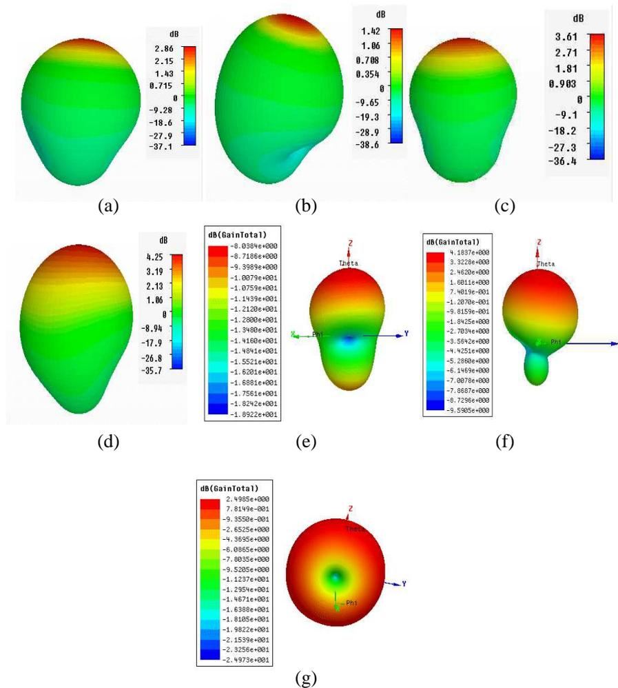
Figure 4. The pattern and gain for 2.45 GHz.
