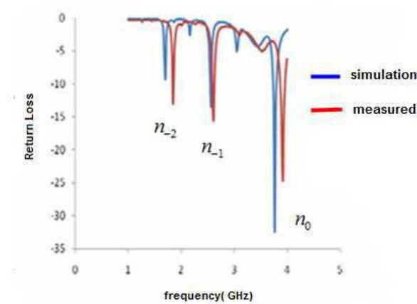
**Figure 7.** Return loss of the first antenna.
