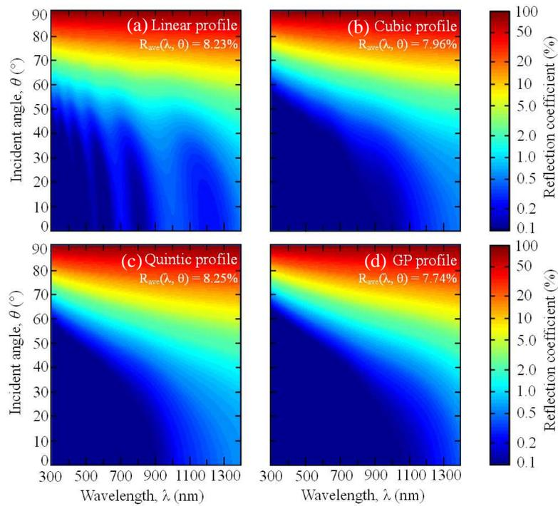
**Figure 8.** Simulated reflection characteristics of  $\text{TiO}_2/\text{SiO}_2$  graded-index AR coating, (a) linear-index profile, (b) cubic-index profile, (c) quintic-index profile, and (d) GP-index profile as a function of wavelength and incident angle.
