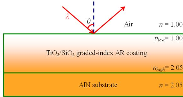
**Figure 6.** Schematic of an 800 nm  $\text{TiO}_2/\text{SiO}_2$  graded-index AR coating between air and an AlN substrate with refractive index of  $n=2.05$ .
