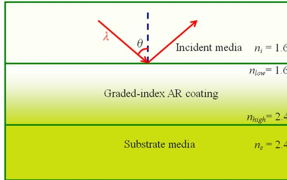
**Figure 1.** Schematic of a 1000 nm graded-index AR coating between incident media and substrate media with  $n_i = 1.6$  and  $n_s = 2.4$ .
