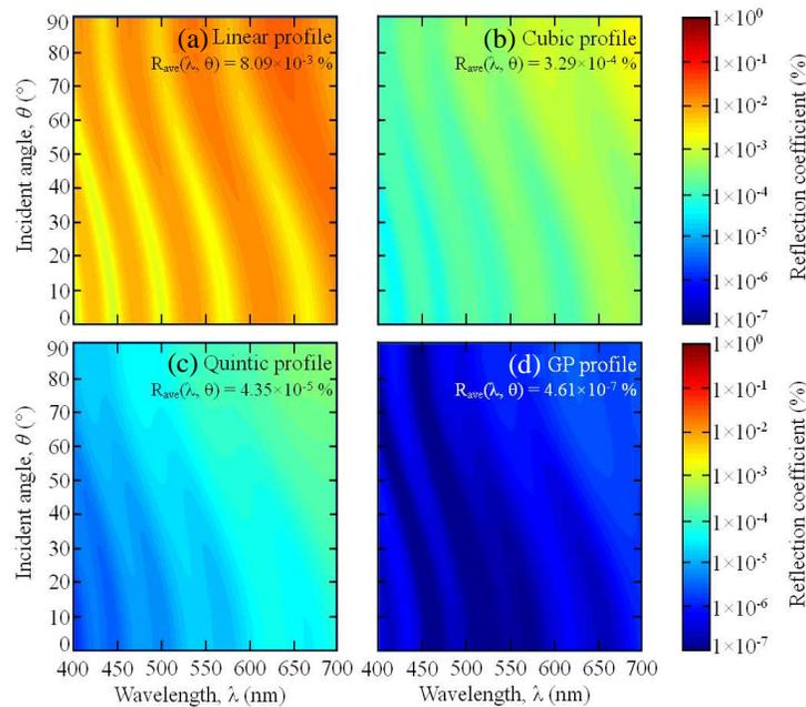
**Figure 5.** Simulated reflection characteristics of AR coatings, (a) linear-index profile, (b) cubic-index profile, (c) quintic-index profile, and (d) GP-index profile as a function of wavelength and incident angle.
