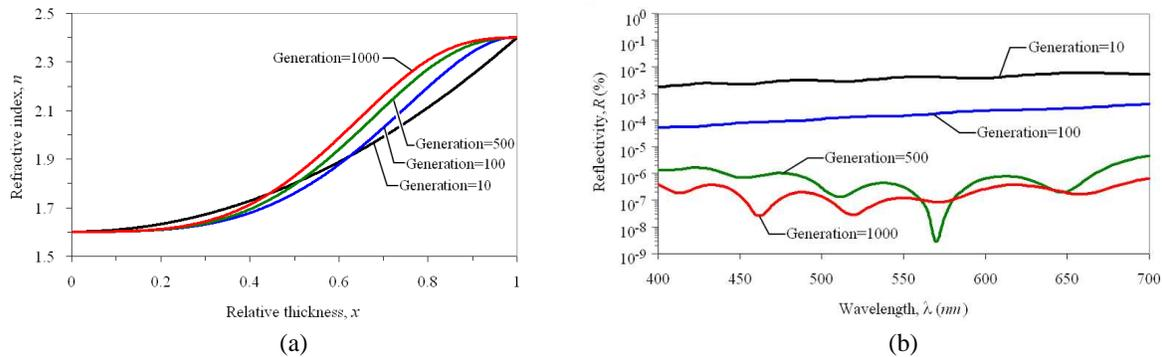
Figure 3. (a) The optimal GP-index profile and (b) calculated wavelength-dependent reflectivity at normal incidence at 10, 100, 500 and 1000 generations, respectively.
