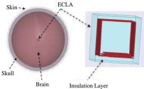
**Figure 4.** ECLA inside three-layer model of human head and magnified ECLA antenna structure.
