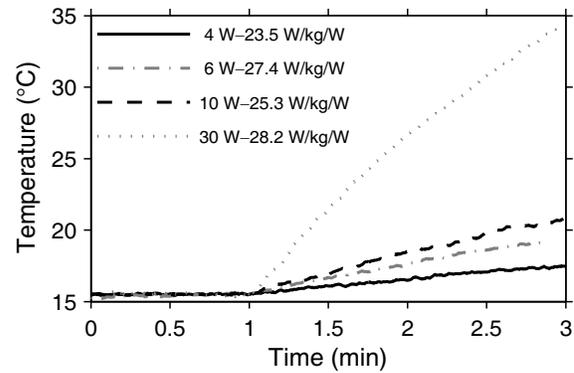
**Figure 6.** Initial temperature rise measured at the position of the optical beams for 4, 6, 10 and 30 W input power (the system is placed in the air conditioned unit and the stirrer is turned on).
