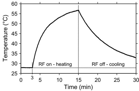
**Figure 5.** Experimental temperature measurements starting at room temperature. The generator is turned on at  $t_{on} = 3$  minutes and turned off at  $t_{off} = 15$  minutes. The input power is set to 30 W and the stirrer is turned on. This temperature measurement is made where with respect to the  $P_0$  position
