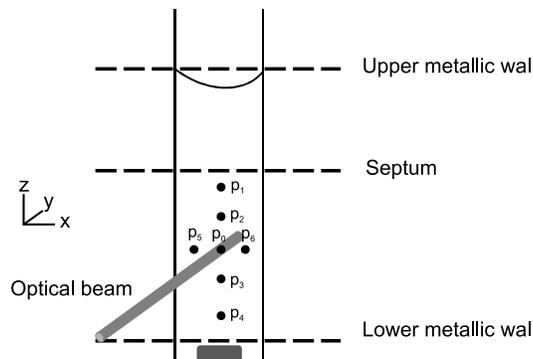
**Figure 3.** Schematic of the cuvette filled with water. The line defines the position of the excitation and emission optical beams. The dots define the positions at which the Luxtron probe was placed for temperature measurements (with a step of 2.5 mm).
