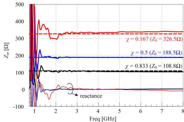
**Figure 5.** Simulated input impedance (solid line) of two-arm planar Archimedean spiral antenna in free space compared with analytical impedance (dashed line) of parallel slotline model by conformal mapping.
