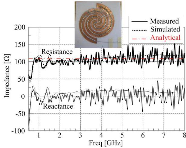
**Figure 8.** Measured input impedance (solid line) after de-embedded calibration of cable, simulated input impedance (dashed line) without the infinite balun, and conformal mapping result (red dash-dot line) of the fabricated spiral antenna.
