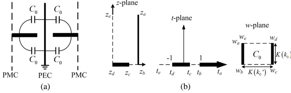
**Figure 4.** Calculation of capacitance  $C_0$  for slotline mode with lateral PMC in free space; (a) equivalent circuit and (b) conformal mapping steps from  $z$ -plane onto  $t$ -plane and then onto  $w$ -plane.
