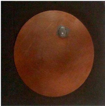
Figure 9. Photograph showing the realized elliptical patch antenna with the dimensions given in Fig. 4.
