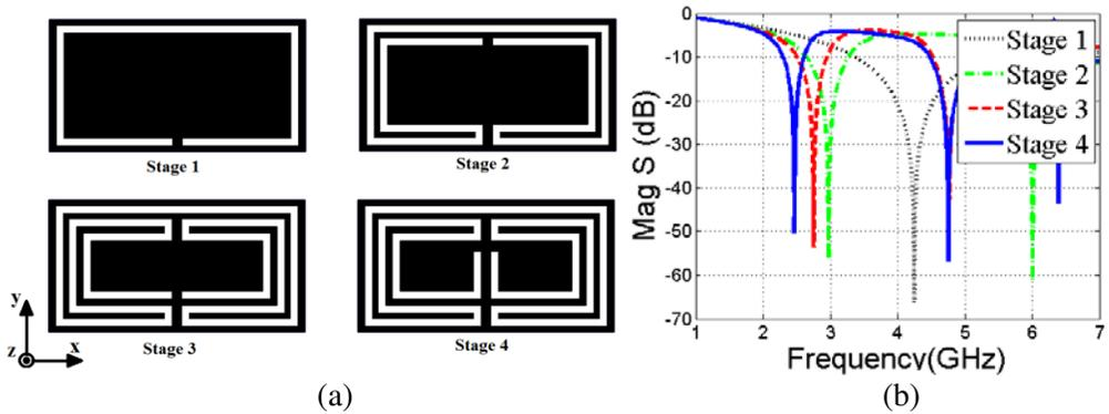
**Figure 3.** Design process of H-IFCSRR (a) geometric stages and (b)  $S$ -parameters ( $S_{21}$ ).
