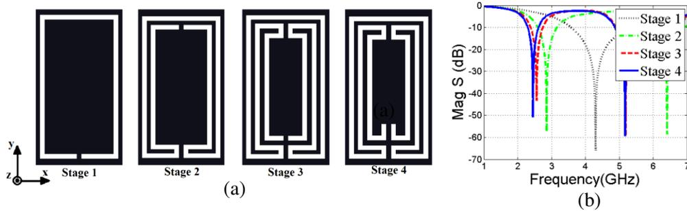
**Figure 2.** Design process of E-IFCSRR (a) geometric stages and (b)  $S$ -parameters ( $S_{21}$ ).
